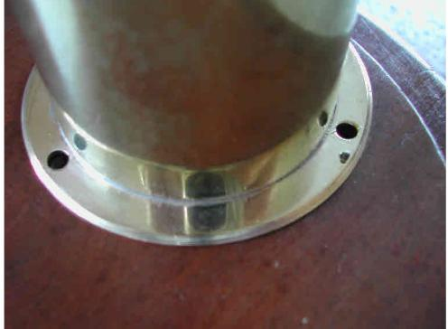
The column does not have a flange and so the brass ring that secures it to the base is soldered with holes for pins to exactly position it on the base.
