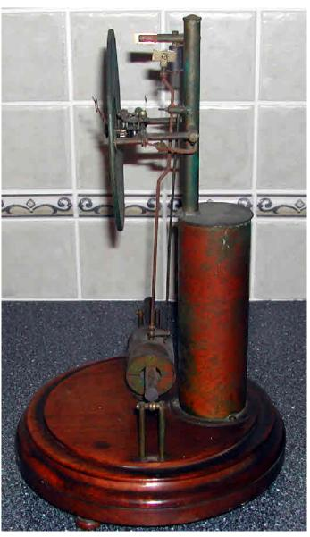
This clock is the earliest Bulle clock I know of an exhibits some very early and rare features. These will be expanded on when the clock is restored. But note the lack of Isochron and Contact springs!. And the damper arm etc.
