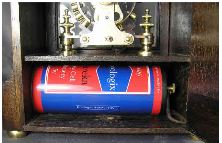
The rear of the restored movement and the replacement “Horologix” regulated battery power supply.
