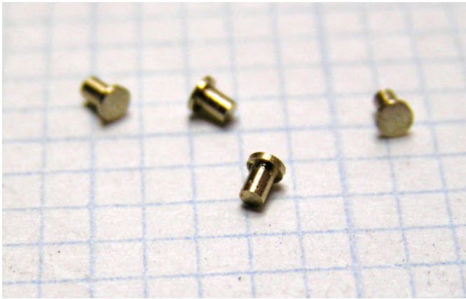
The rivets after filing. They are now ready to be fitted.
