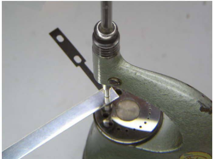
The Parts being riveted together in the stake. The photo below shows the flag spring immediately after riveting The second flag shows the situation after being roughly trimmed to shape ready for chamfering the edges with a needle file.
