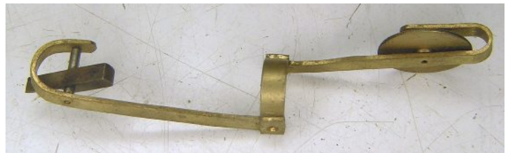
Above is shown the second type of impulse arm normally found on Eureka clocks. They can be of a two part design screwed together or, as in this case, formed from a single piece of brass bent and formed into shape.
