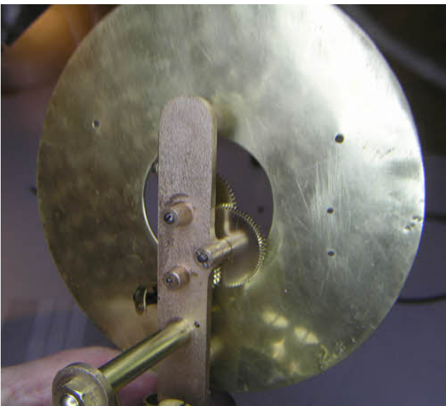
The final missing part was the frame nut which has now been replaced.
