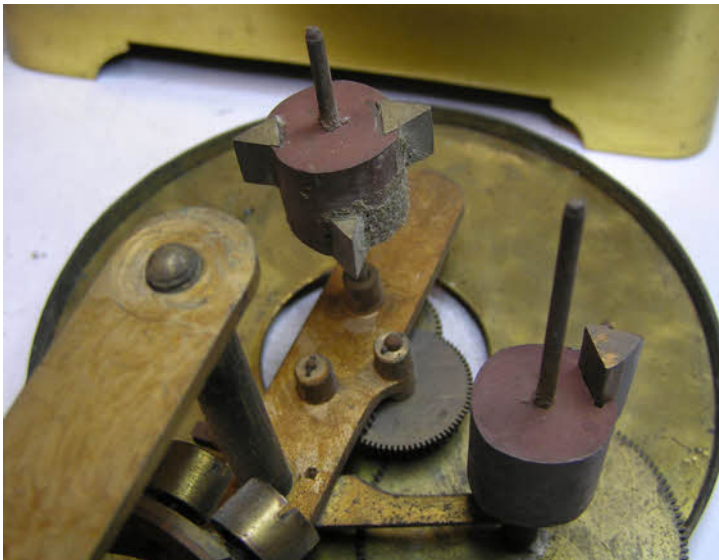
Note the one triangular brass insert in the arbour driven by the motion work.
