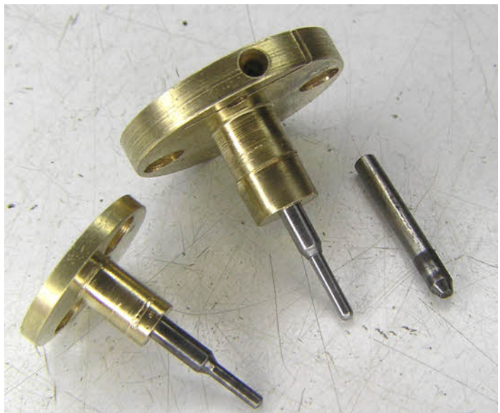
New front pivot polished and in place.
