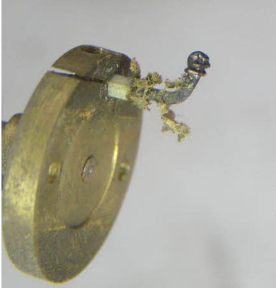
The contact pin assembly had started to disintegrate.
