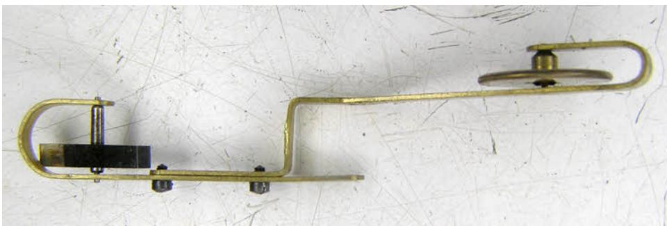
The click spring for the count wheel looks too good to be true. It looks as though it may have been replaced at some point.
