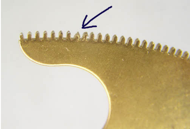
Even the quadrant has not escaped damage. Note the bent teeth (arrowed). I will straighten these relatively easily with a little care.
