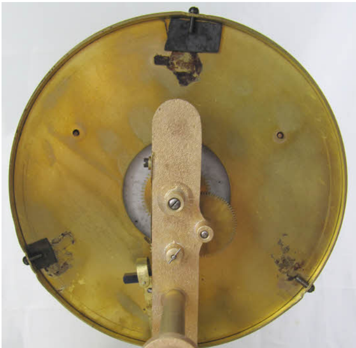
The rear of the dial shows some bad marks and some padding where the screws are not holding the enamelled dial tight the dial pan. I'll investigate and remedy this.
