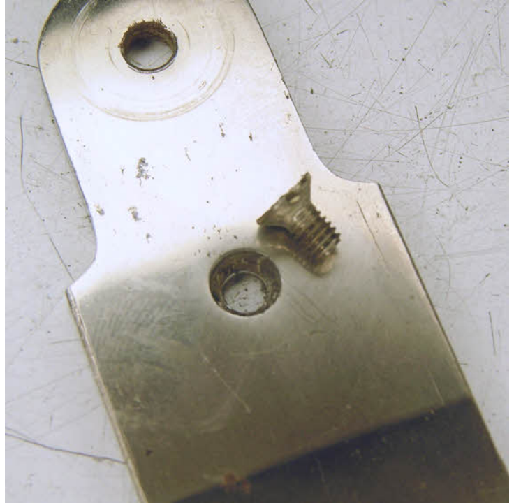
The screws that secure the base plate to the pillars are wrong. They should be shouldered cheese heads. I will turn some up on the lathe.
