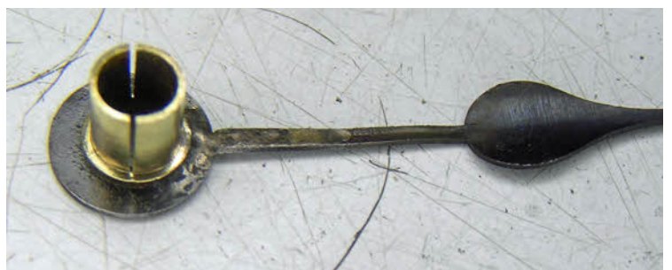
The hour hand had a silver solder repair which is hardly noticeable from the front so it was left as is.
