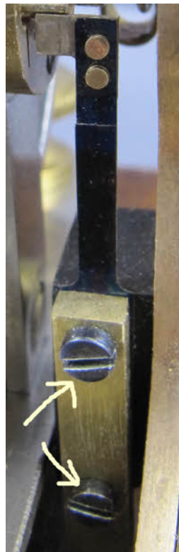
These two photos shows the position of the motion click spring and a close up of the damage caused by the constant wearing of the count wheel teeth. It has worn completely through and will need replacing.
