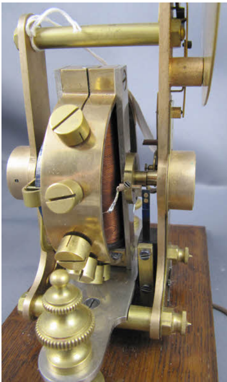
These two photos shows the position of the motion click spring and a close up of the damage caused by the constant wearing of the count wheel teeth. It has worn completely through and will need replacing.
