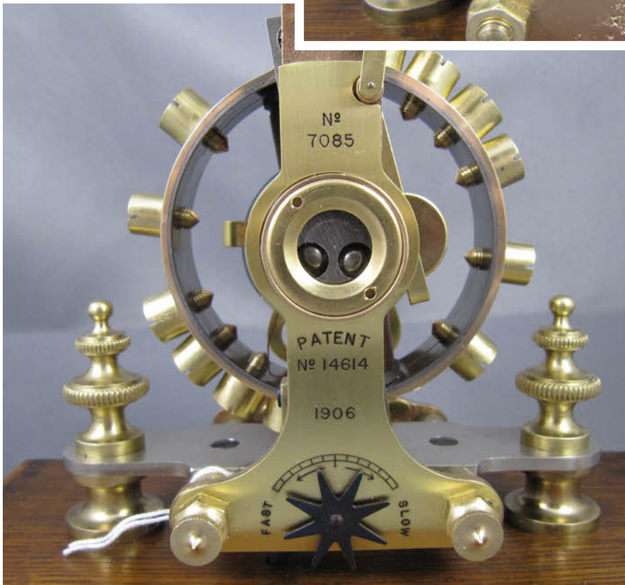
These two photos show the finished front and rear bearings. Note the registration plate engraving has been wax filled and the then polished and lacquered.
