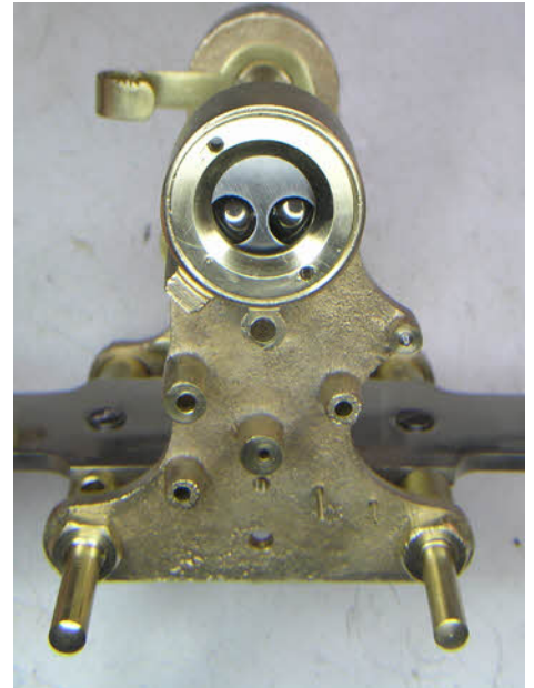
At left we see the balance wheel after repair. The contact pin now needs to be soldered in place. Above is the rear bearing after cleaning.
