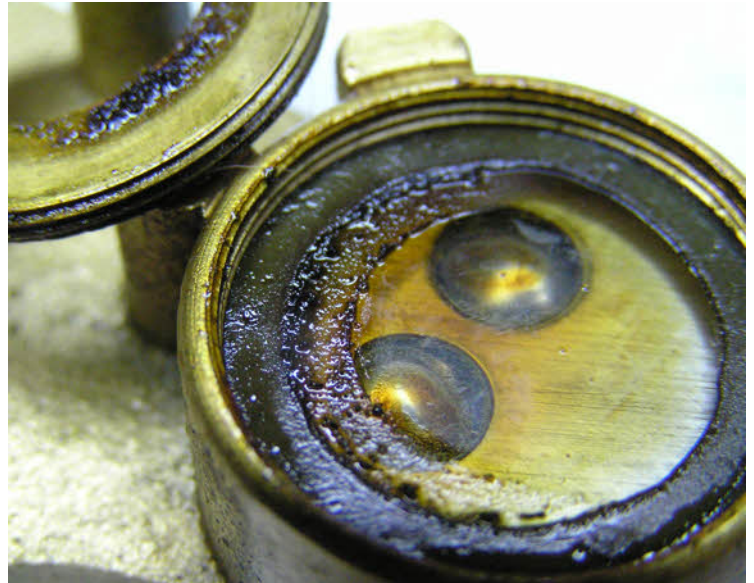
The grime in the rear bearing housing turned out to be caked oil; thank goodness. This is a lot easier to treat than rust.
