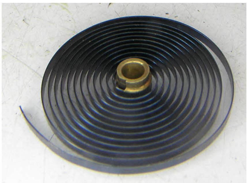
This photo shows the new stop spring after initial cutting out from 0.004" spring steel. It just needs final shaping before fitting.
