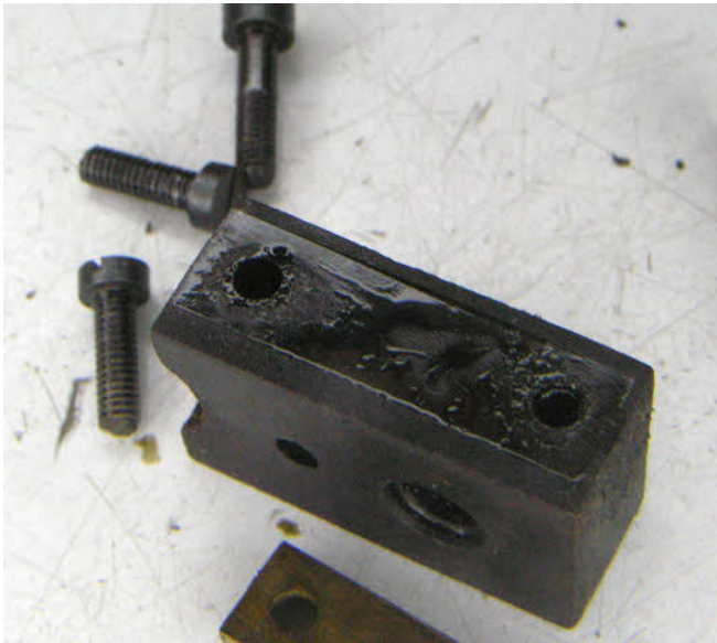
The contact flag insulating block is covered in oil and wouldn't have been good for the electrical contact. It should clean up OK .
