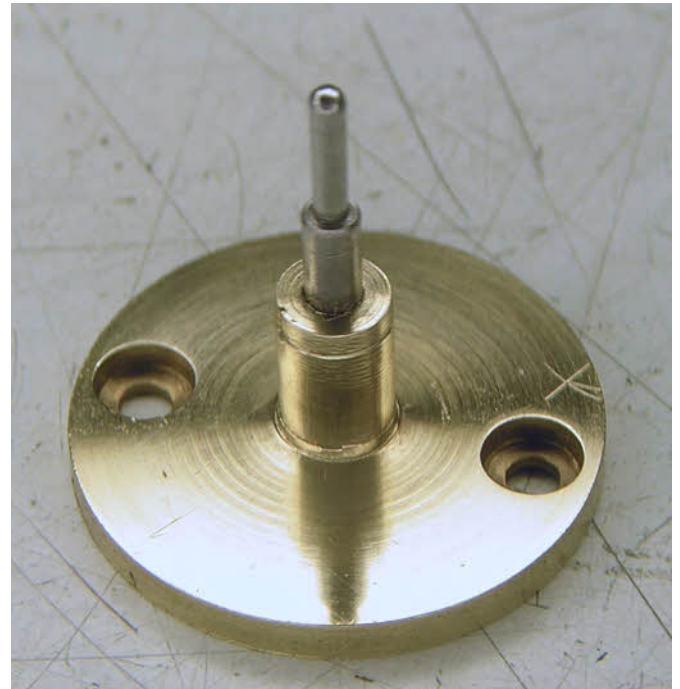
These photos above show the new pivot secured into the rear pivot housing.
