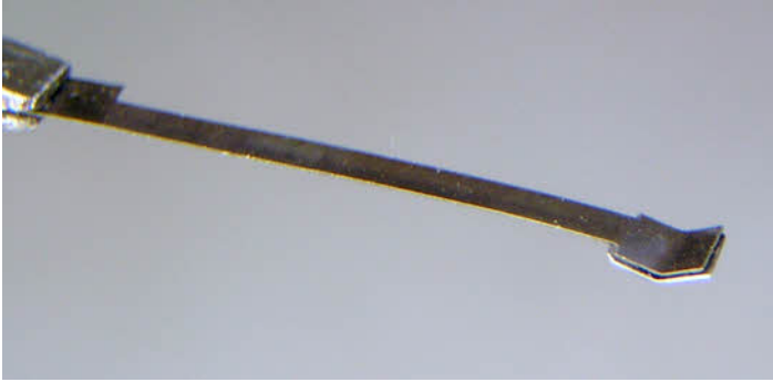
The spring with the new piece soldered in place ready for grinding the side flush. This is a neat repair and saves as much of the original as possible.
