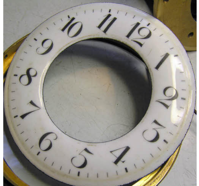
The dial front and back. It is in near perfect condition with just some dirt and grime around the edges which is easily cleaned with warm soapy water.
