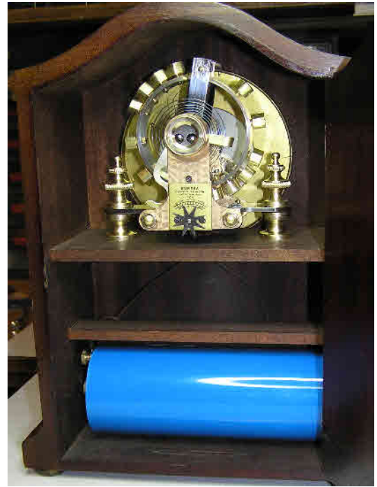
Photos of the re-assembled clock. Note the replacement flag cell battery fits perfectly in the original housing.
