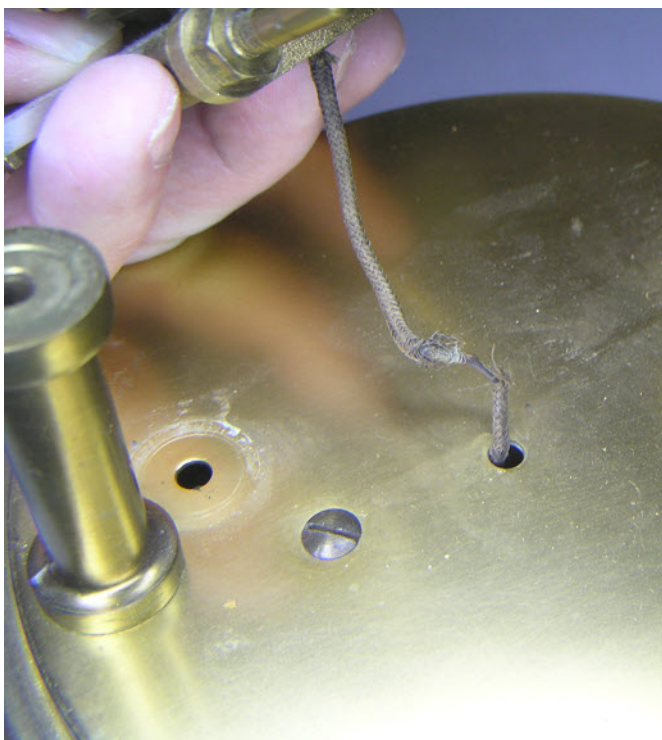
The positive lead has been cut nearly through and will need to be replaced.
