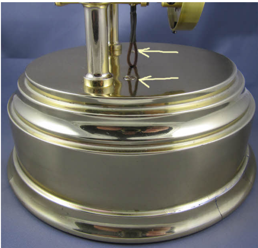
The photo below shows the finished base and counter-sunk screws.
