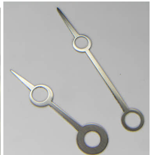
The new moon hands ready for blueing and mounting on collets.
