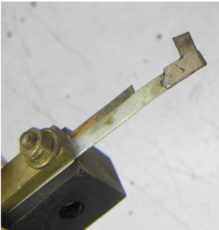
This photo shows that the flag contact assembly is a home made piece of spring steel with a piece of silver soldered in place. The block to which it is attached looks to be damaged with two large nuts and bolts holding the flag in place. The whole assembly will need replacing.
