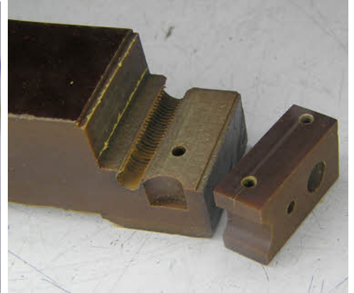
The new contact flag block cut from the solid and with the new flag below.
