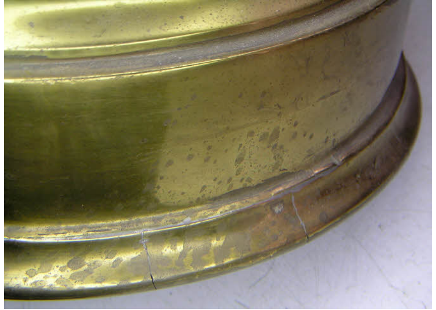
This photo shows the outside of the base where the brass has been reinforced. There are solder burn marks but these should polish out OK. But the joints will still be noticeable.
