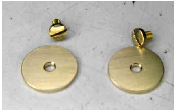
The new dial washers to be fitted to the back of the dial.. Below and below left, we see a side view of the finished clock.
