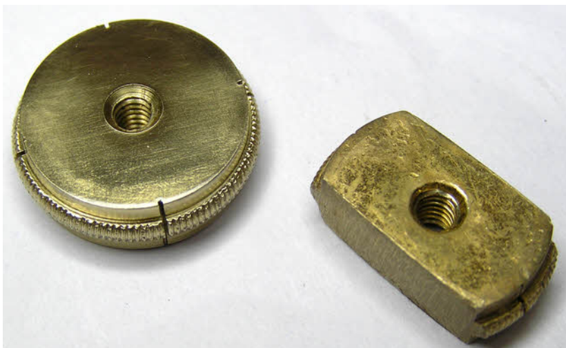
Above we see the cut up rating nut on the right and the replacement on the left.
