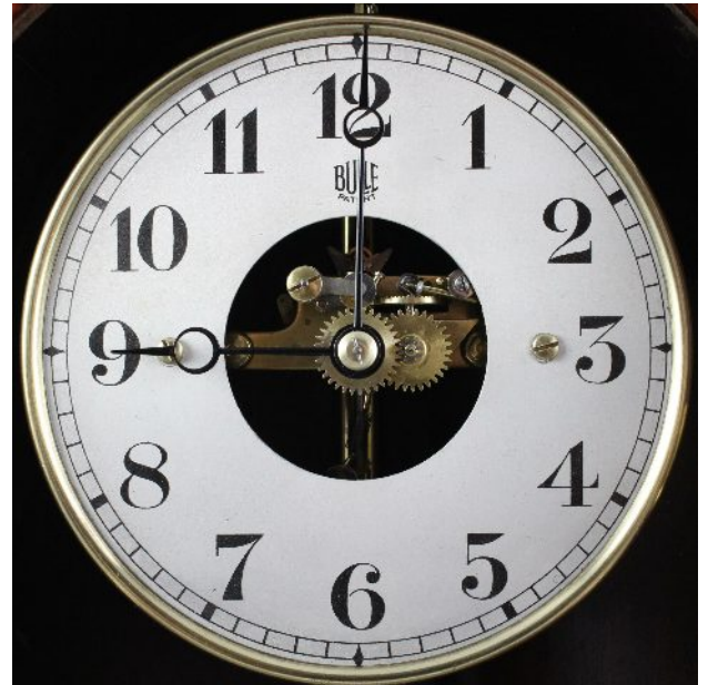
The photo on the left shows the case after gluing the various fractures and lifted veneer. A stain has then been applied followed by a sealer and about four coats of French Polish. The photo above shows the cleaned dial back in place with the restored hands and replacement collet.
