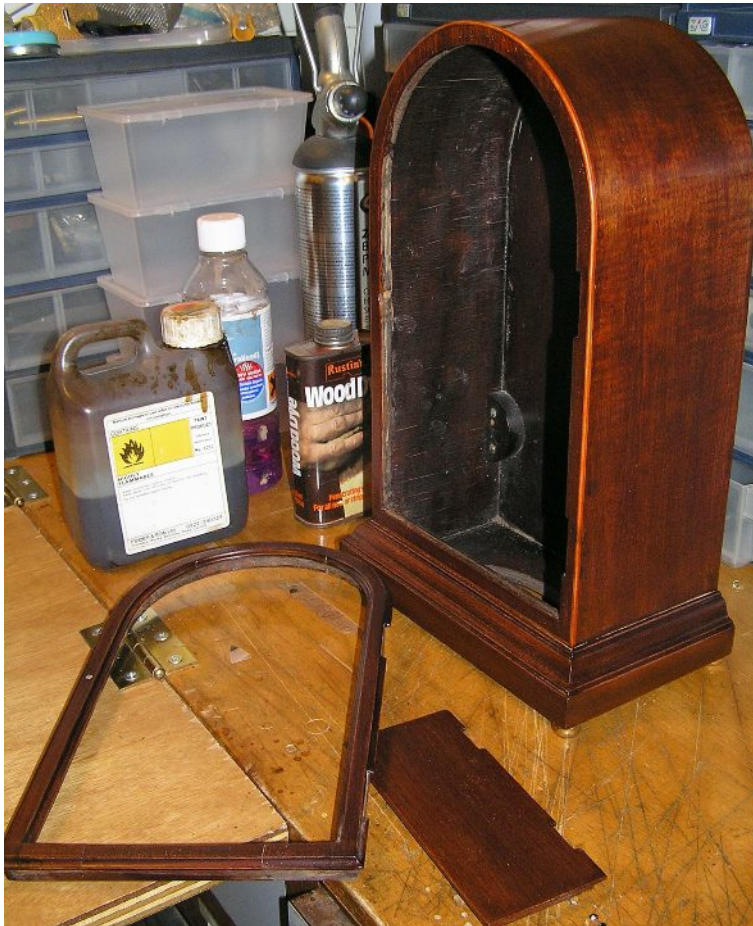
The photo on the left shows the case after gluing the various fractures and lifted veneer. A stain has then been applied followed by a sealer and about four coats of French Polish. The photo above shows the cleaned dial back in place with the restored hands and replacement collet.
