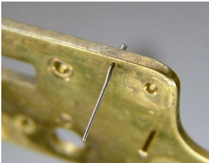
This looks to be a spring [in from a French clock. Why it is here is a mystery. There is a perfectly good pendulum stop pin to its lower right.
