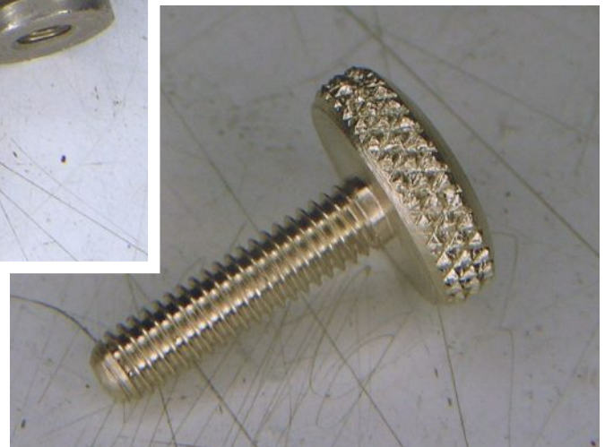
At right is the new case levelling screw turned up on the lathe.
