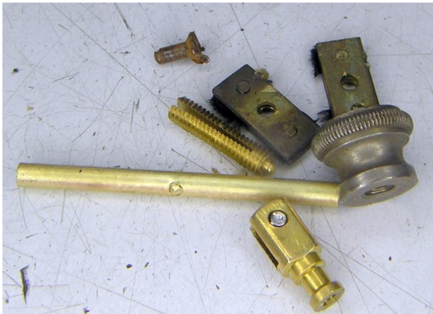
At right is the new case levelling screw turned up on the lathe.
