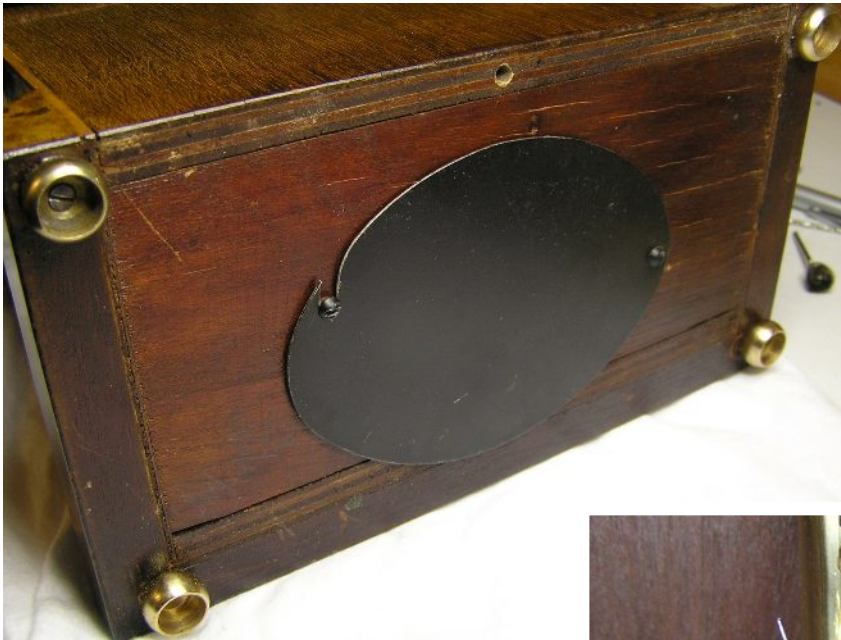
Above is the base of the case with the Barometer dial cover. Top right I sthe new levelling screw in place.
