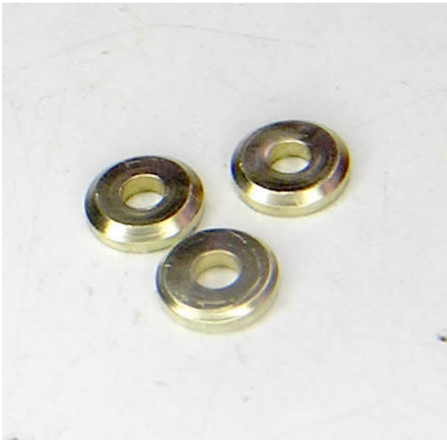
The three spacing washers required to finish the movement. The first was used on the pendulum contact assembly shown in the photo on the right. The other two were used to correctly space the movement onto the frame.
