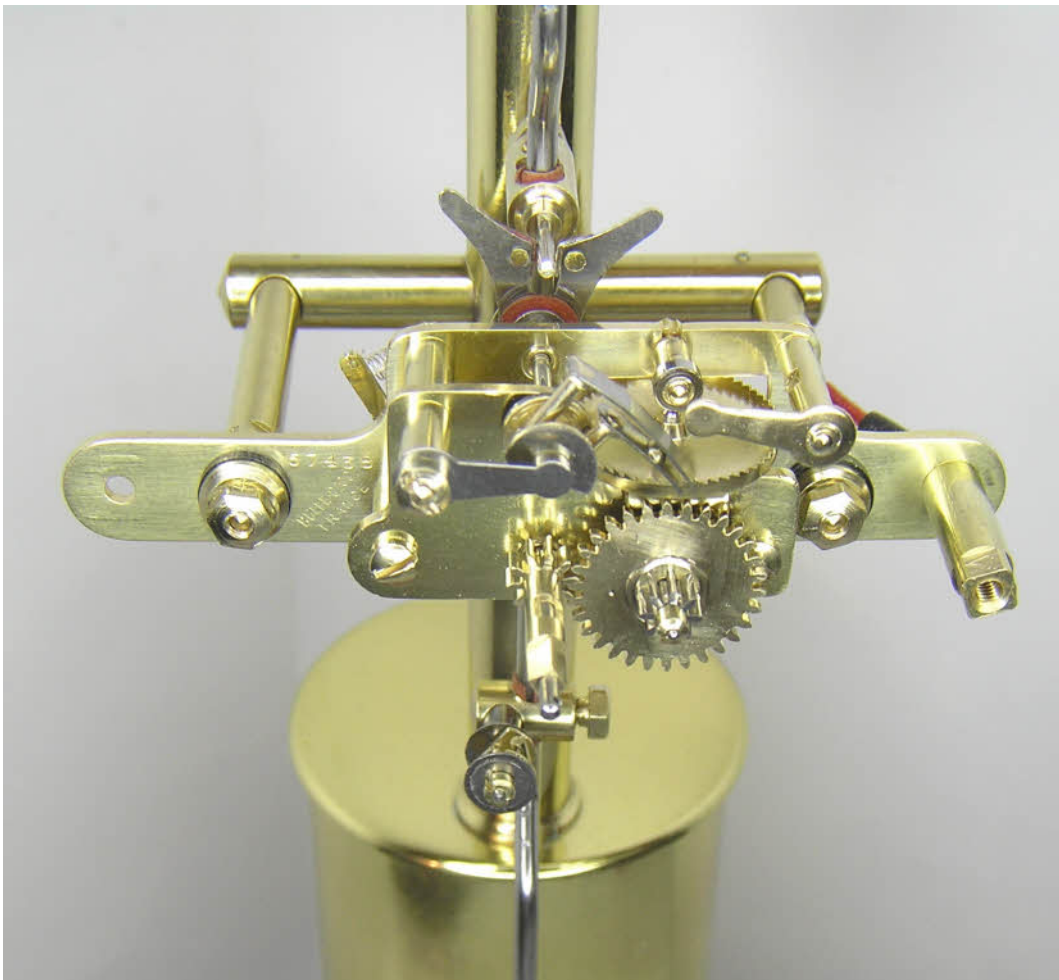
The movement mounted in the frame with the pin positioned in the fork.
