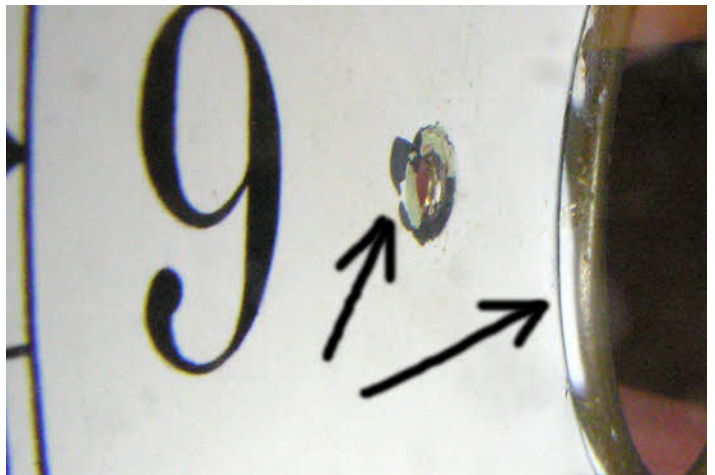
The dial has been repainted as can be seen from the over-spray marks on the brass (arrowed). The execution is excellent though perhaps a little flakey. We will have to be extra careful when cleaning the inner and outer brass rims.
