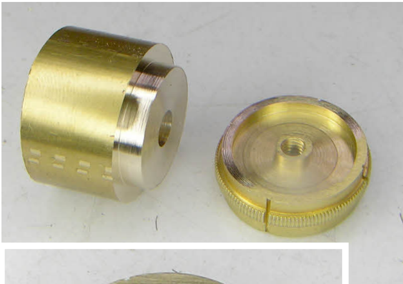
The insert ready to be inserted and machined flush.
