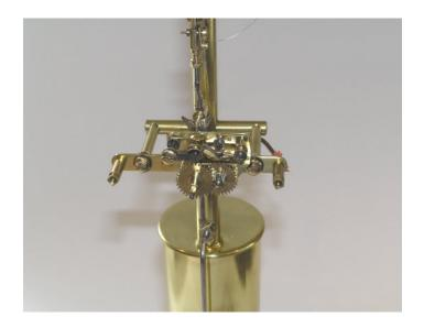
The original wiring was in a bad way and had to be replaced. Sometimes you can recover the wire if it has not deteriorated to badly. But if the copper core is corroded then you have no choice. In other cases it is possible to re-use the cloth covering by removing the copper wire and re-threading new. But this is a tricky process.
