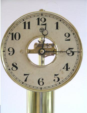
The brass dial surround is hard to clean because it is crimped around the insert during manufacture and bends round into contact with the face. I use a thin brass shim cover which inserts under the rim whilst cleaning with "0000" gauge wire wool. The hands have been cleaned and blued. They really set of the dial. The <u>Suspension</u> is a Horologix replacement.
