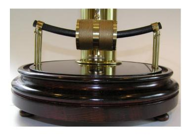
The <u>Silver contact</u> spring was missing on this clock and I have fitted a Horologix replacement. I realised that I had the original Isochron spring so this has been re-fitted
