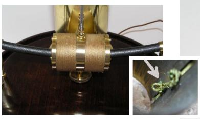
It always strikes me as odd when I do these clocks that in 90% of the cases the cord has faded to the same degree all round the pendulum regardless of whether it has been in direct sunlight or not. The cord on this one has faded to a lovely golden straw colour. Unfortunately it makes it very difficult to clean and polish the Brass around it. One has to resort to "Q" tips.
