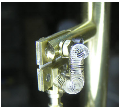
The two photos above show the detail of the box tube and the screwed pin which is the arbour for the intermediate minute wheel.
