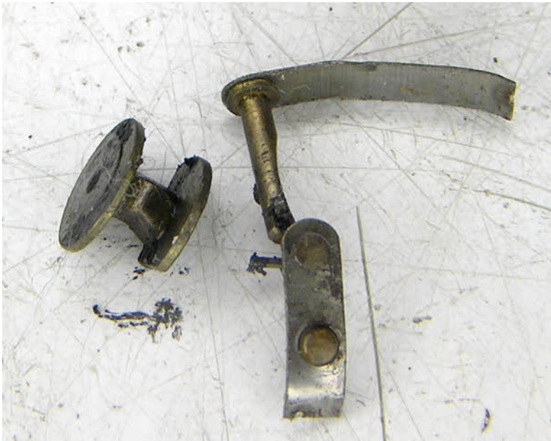
These two photos shows the amount of oil sludge present in the pawl assembly and the count wheel. But it is easily cleaned up.
