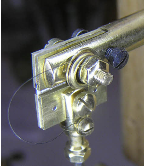
The new silk suspension with the original contact wire.
