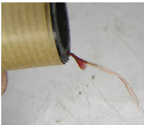
The photo at left above shows that the hole did not penetrate right though to coil and I was able to remove the old paper and secure the loose coil loops with new paper. The coil ends were also cleaned and readied to receive new wire extensions.
