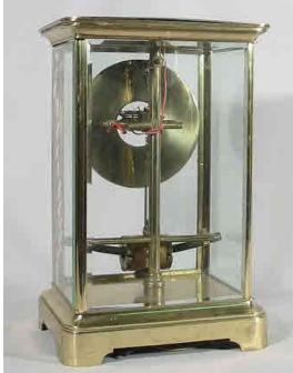
Nice Four Glass Tall Bulle clock. It has had new wiring in the past, but other than that it looks as though it is untouched. I replaced the broken suspension with a new one. The case is in good condition although the lacquer has worn away in places. The coil still retains the original cord which has aged gracefully to a straw yellow. The dial is of the aluminium insert type and is in excellent condition.
