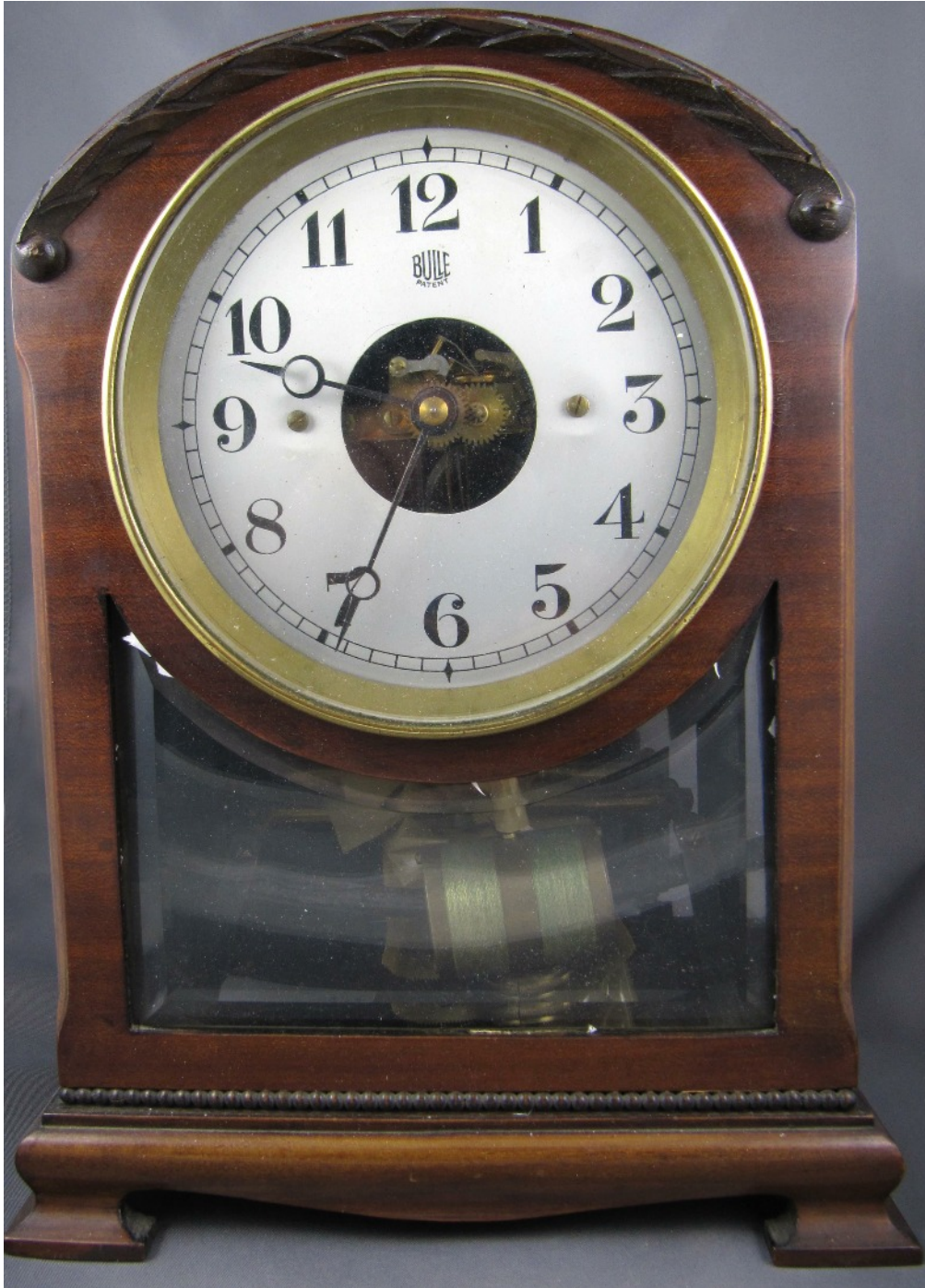
Photos by kind permission of the owner. A medium movement Bulle with a 0.44 beats per second pendulum in a mahogany veneered case with opening bezel, bevelled glass panel and rear door. Overall the clock looks in good condition with the case just needing a good wax polish although there is an old stress crack on the top of the case.
