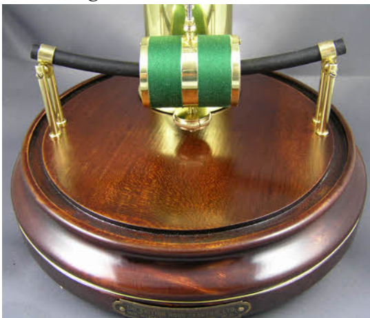
The coil back in the cover with pendulum rod and rating nut.
