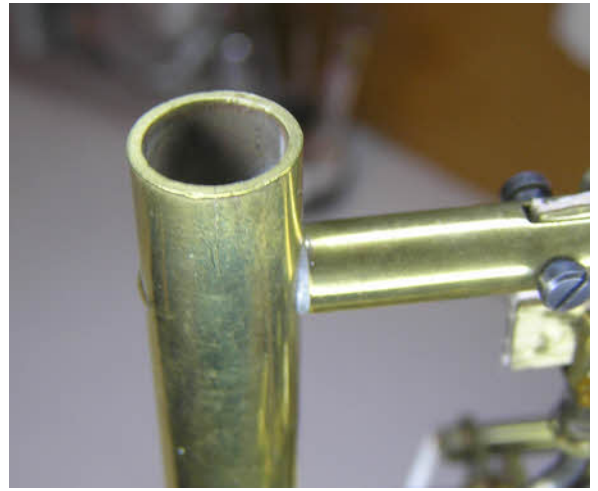
Two photos showing the corroded brass decorative wire and the top of the frame tube.
