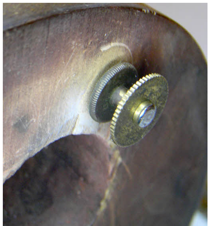
The photo left above shows the corroded battery compartment cover with missing brass knob. The photo above shows the third levelling foot which has a knurled extension added to compensate for the fact that the original screws has worked loose over the years and will fall out of the wood if unscrewed by more than a millimetre or two. This will be corrected. The photo as left shows the corrosion inside the tube.
