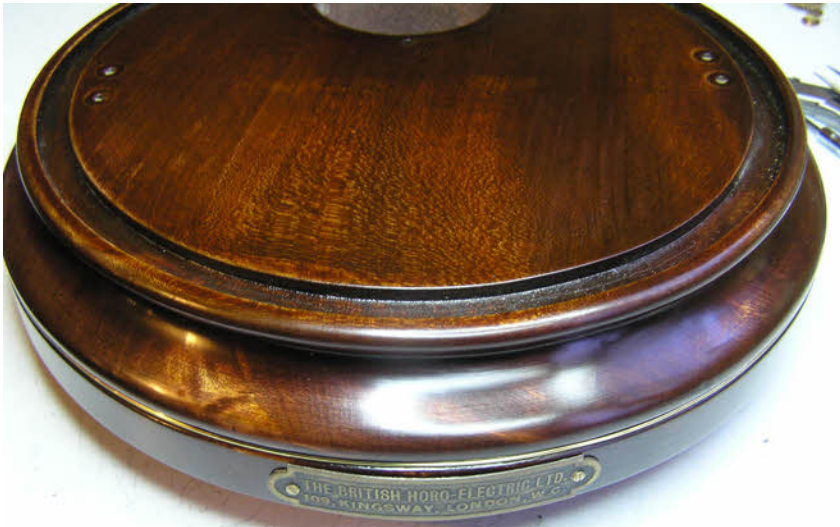
The polished base with new decorative 1.00mm brass wire, and the restored levelling screw back in place
