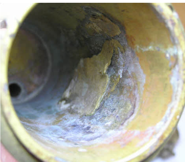
The photo left above shows the corroded battery compartment cover with missing brass knob. The photo above shows the third levelling foot which has a knurled extension added to compensate for the fact that the original screws has worked loose over the years and will fall out of the wood if unscrewed by more than a millimetre or two. This will be corrected. The photo as left shows the corrosion inside the tube.
