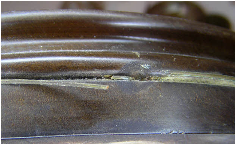
Two photos showing the corroded brass decorative wire and the top of the frame tube.
