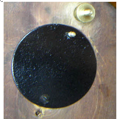
The frame ready to accept the movement. Note the stepped red fibre insulating washers. On these early clock is usual to see red stepped inner washers with black plain outer washers.
