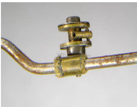
The silk suspension unit is missing and has been replaced with a steel spring. The special screw and nut have obviously gone with the suspension and a standard screw and nut used instead. The missing parts will be turned up on the lathe.
