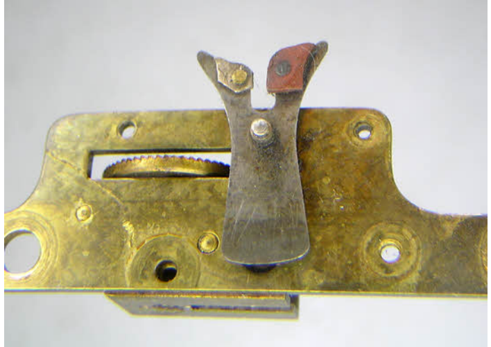
The fork has obviously had some attention in the past with a new piece of fibre added at some point. The silver contact also looks like a replacement. The fork arbour and fork itself look OK.
