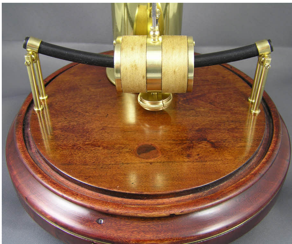
The base with magnet and pendulum . Note the 1/2 inch plug fitted at some time into a drilled hole. I still can't think of a reason for it be there. Still it's a part of the clocks history and doesn't detract from the aesthetics of the clock.
