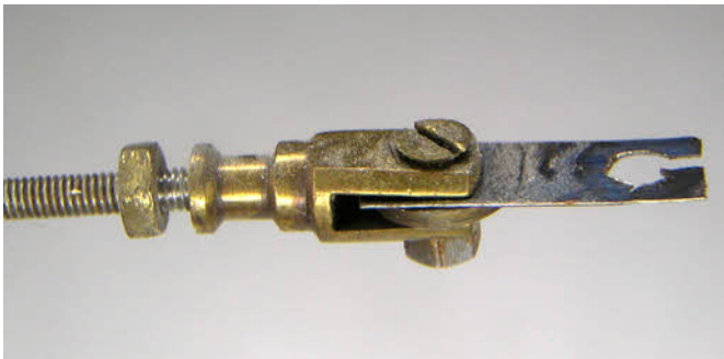
The silk suspension unit is missing and has been replaced with a steel spring. The special screw and nut have obviously gone with the suspension and a standard screw and nut used instead. The missing parts will be turned up on the lathe.
