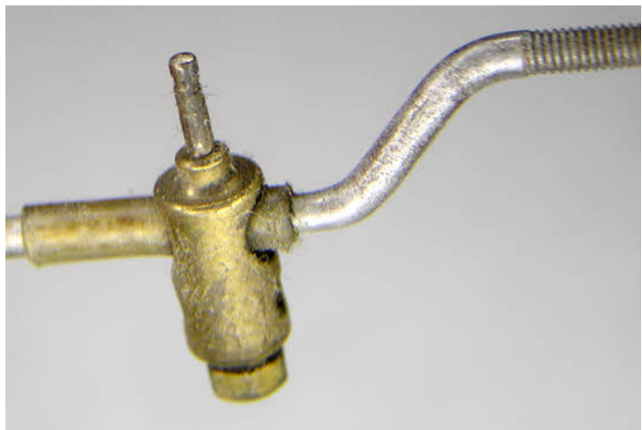
The contact pin assembly is missing the original fibre insulating sleeve. A piece of plastic tube has been used instead. The original fibre will be replaced.
