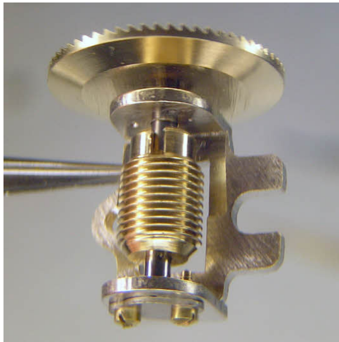
The cleaned worm wheel assembly.
