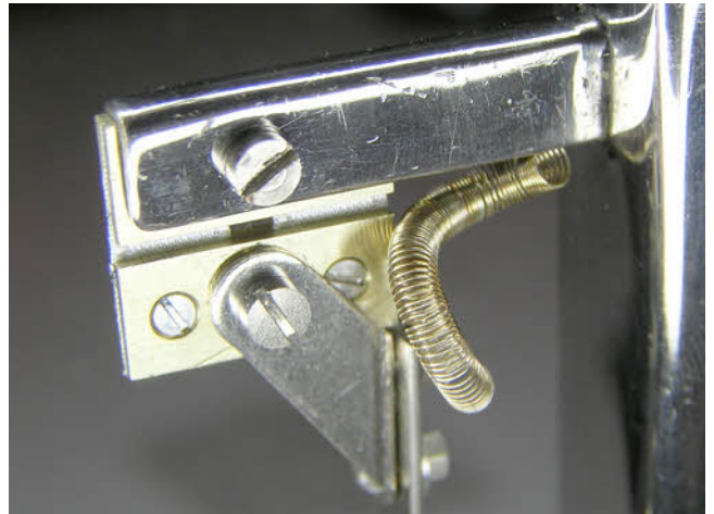
The waxed base with the restored pendulum in place. Note the new suspension and coil.
