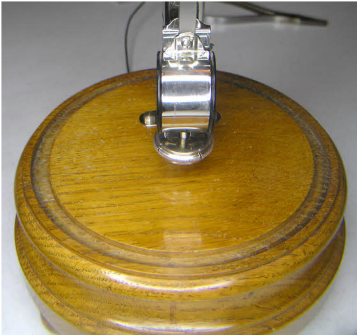
The waxed base with the restored pendulum in place. Note the new suspension and coil.
