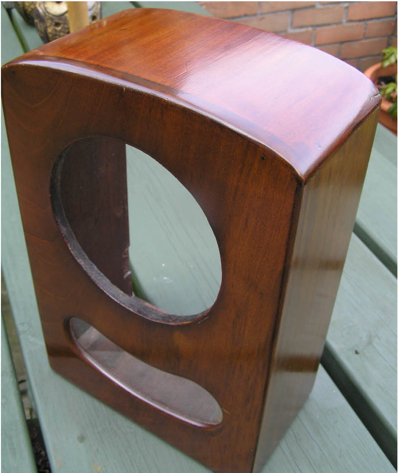
The case after gluing, cleaning, staining and polishing the top. I haven't gone overboard in trying to hide the repair. I didn't want it all to look brand new.
