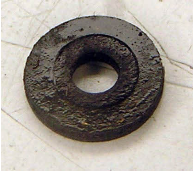
The oil on the fibre washers is in complete contrast the rust evident elsewhere on the steel work.
