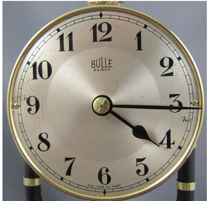
Note the rust has easily been removed and the new minute hand manufactured.
