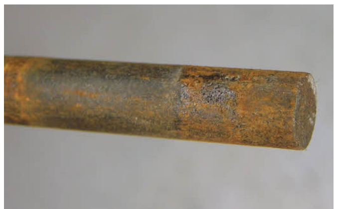
The steel screws securing the feet are badly corroded and will be replaced, if I can get them out! The magnet is also quite rusted but will be easily cleaned and restored with fire grate paint.
