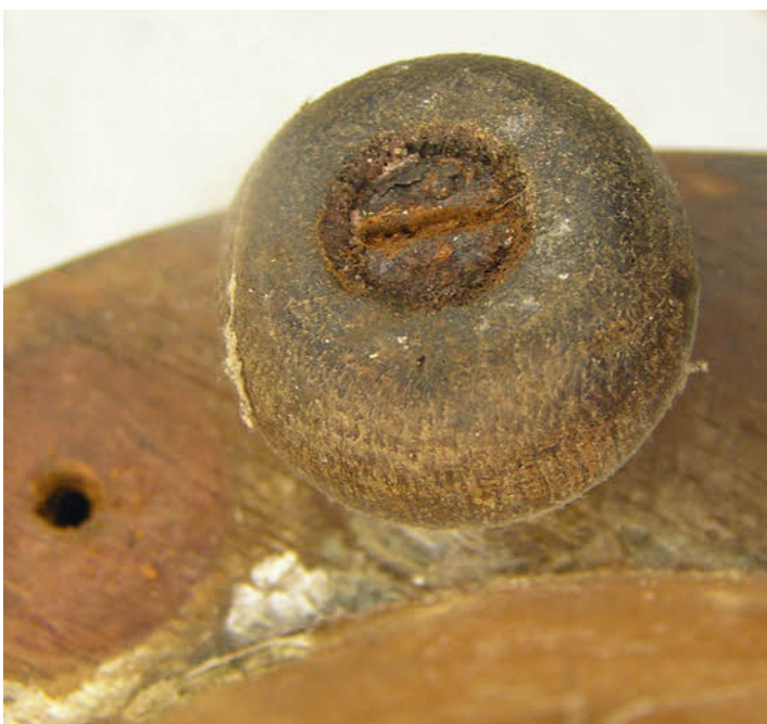
The steel screws securing the feet are badly corroded and will be replaced, if I can get them out! The magnet is also quite rusted but will be easily cleaned and restored with fire grate paint.
