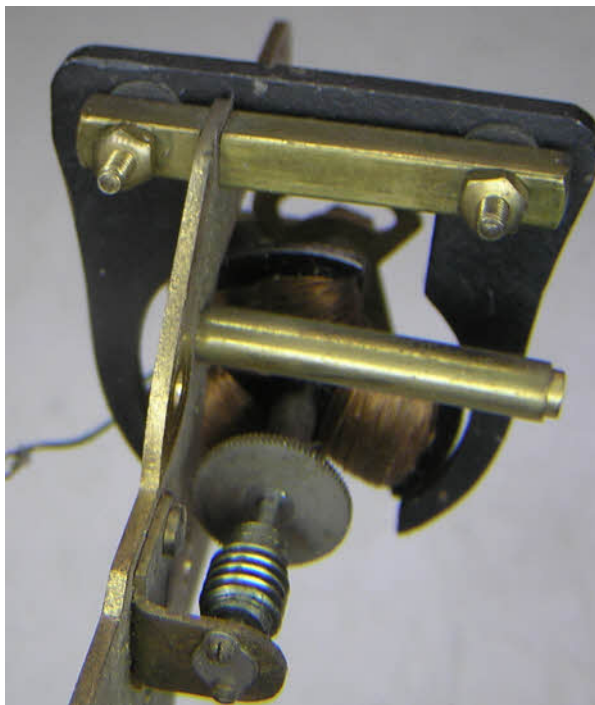
The photo on the right shows the broken fork arbour and the extra parts needed to hold the intermediate motion wheel that carries the half hour and hour lifting pins.
