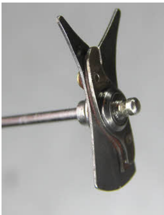
Above and left are photos showing the broken fork arbour and its new replacement.
