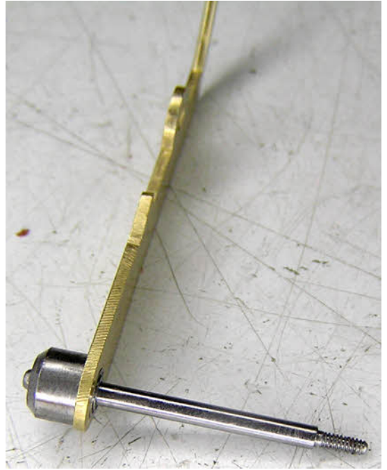
This group of photos above show the damaged arbour and new replacement.
