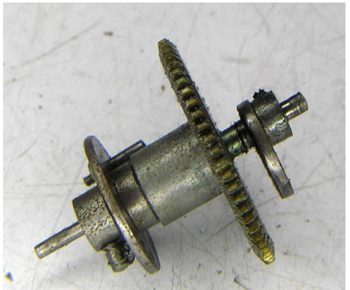
The hammer lift arbour. The wheel is driven by the worm wheel on the motor arbour.
