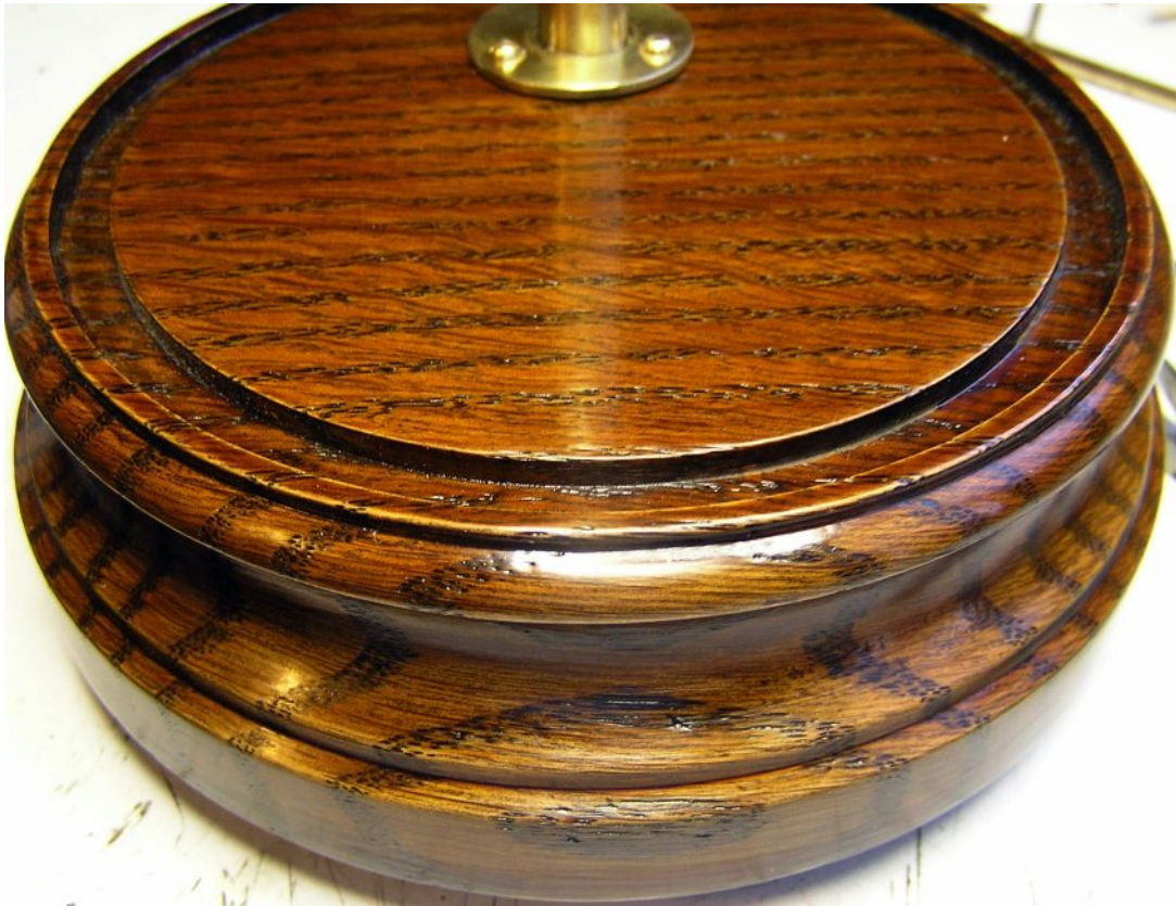
Here we see the base after staining and polishing. The colour is a good match for the original.
