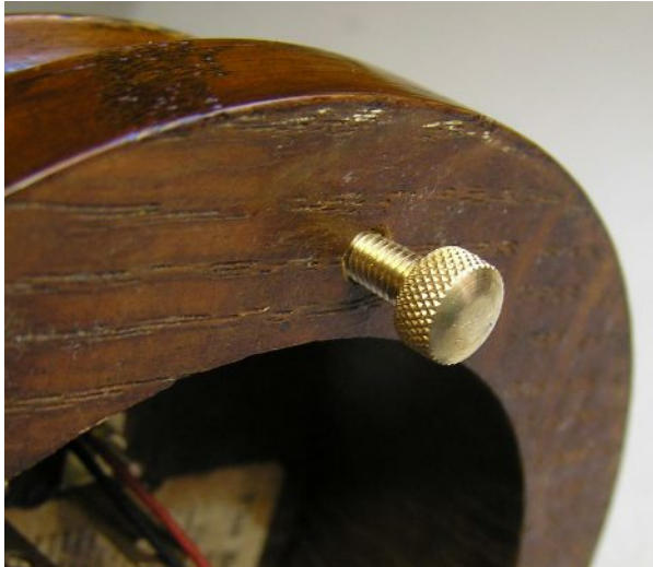
The cleaned base steady screw cleaned and back in place.
