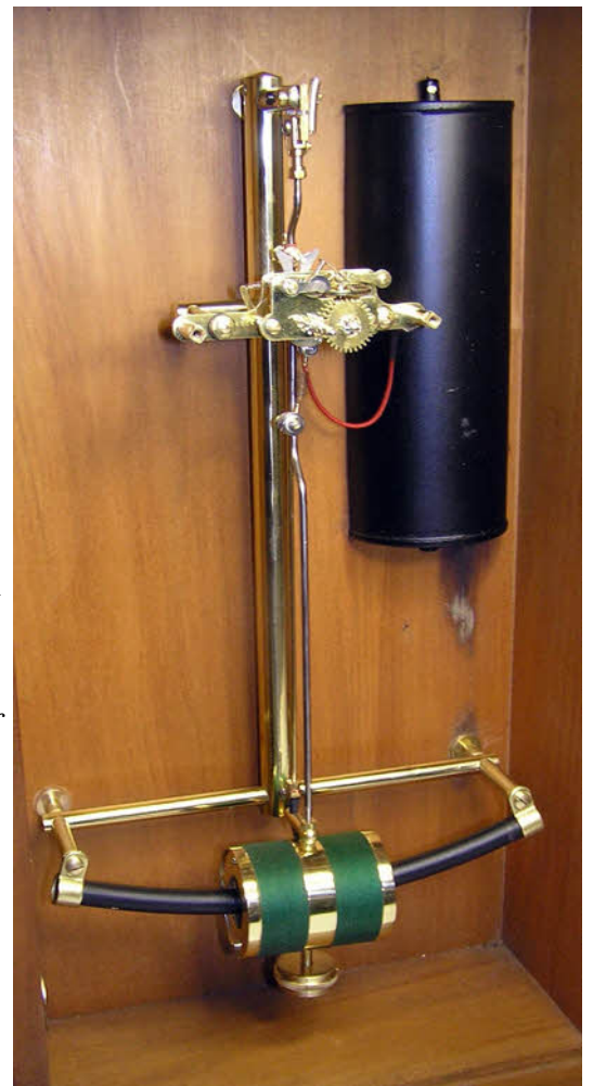
These photos shows the clock back in the case with new coil binding. Note that the battery housing has been damaged through acid leakage, although it shouldn't get any worse after I cleaned away all the acid and gave it a protective coat of paint.
