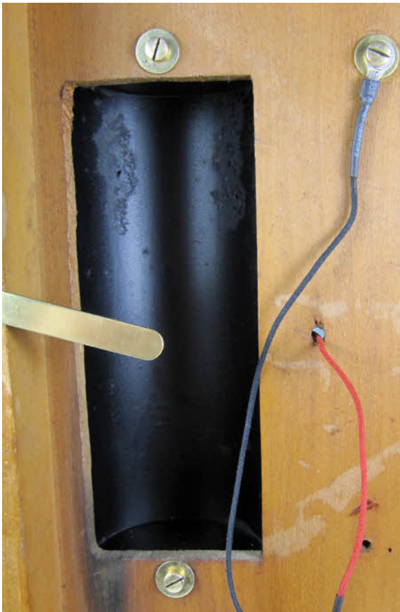
These photos shows the clock back in the case with new coil binding. Note that the battery housing has been damaged through acid leakage, although it shouldn't get any worse after I cleaned away all the acid and gave it a protective coat of paint.
