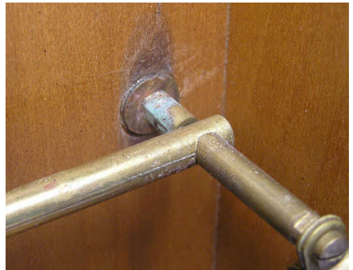
The photo above shows the lead out wire from the pendulum has no insulation and will short out on the brass. The insulation is old and dried right out. It crumbles when touched. The last photo shows the corrosion on one of the stand off pillars.
