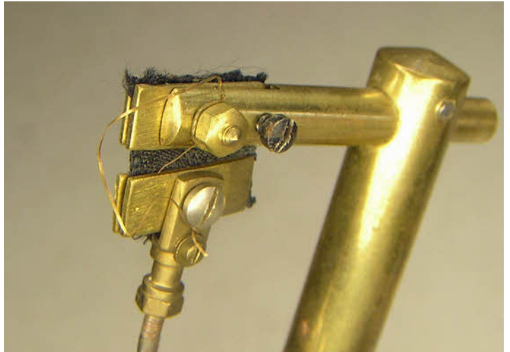
The replaced suspension and contact wire. Both will need to be made.
