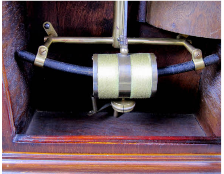
The cord around the pendulum case looks to be a little the worse for wear. On examination it was found to be glued down in places where it had frayed and separated from the casing.
