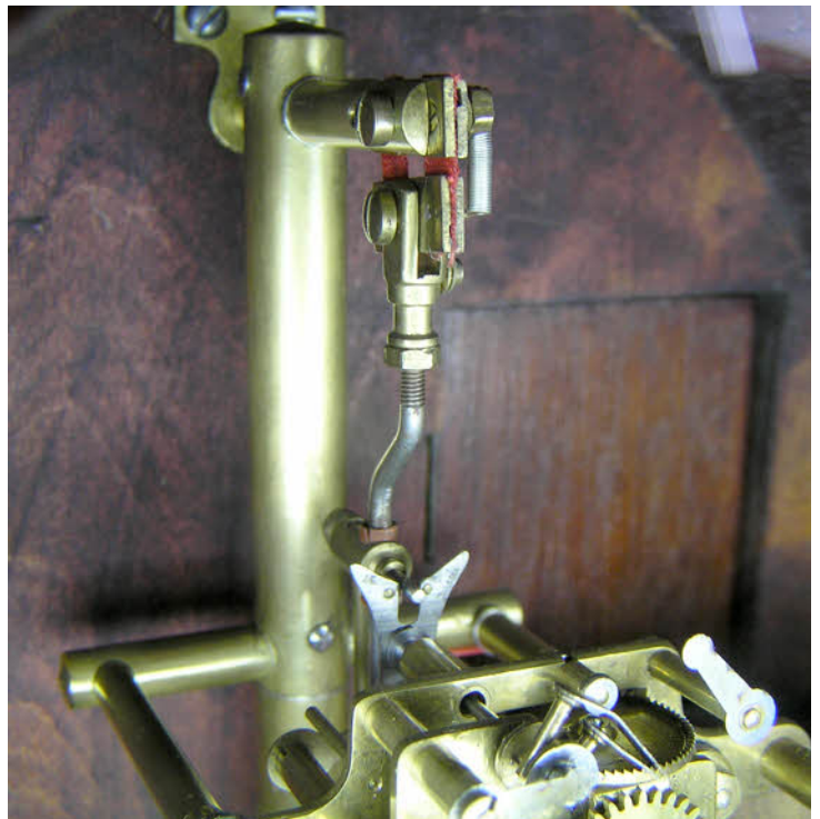
The only issue seems to be the suspension unit which will be replaced.
