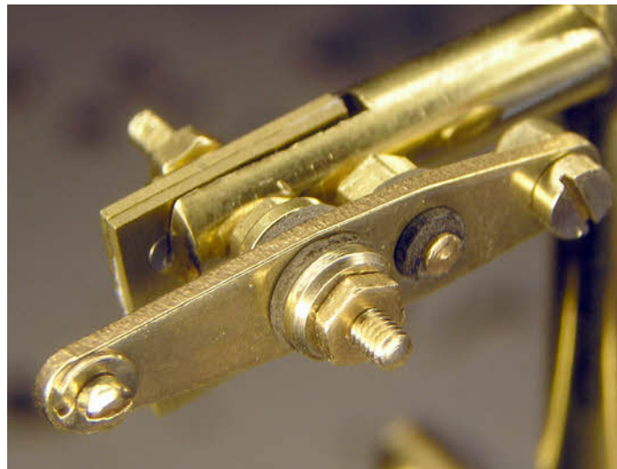
The isolation bar back in place with new screws , nuts and washers.
