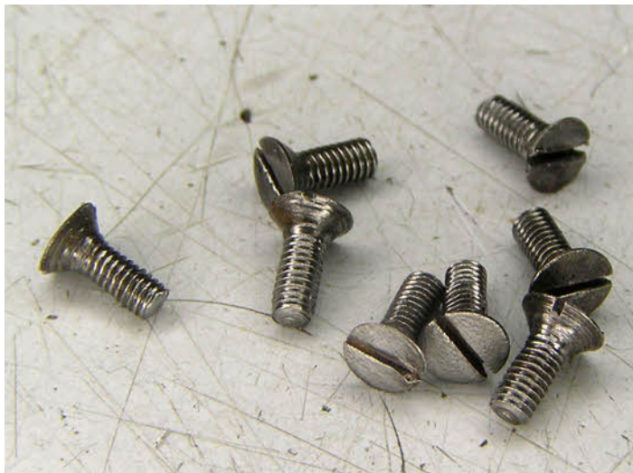
The group of screws that hold the brass case together after cleaning.
