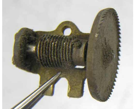
The worm and count wheel are dirty with some rust. But they should clean up well.
