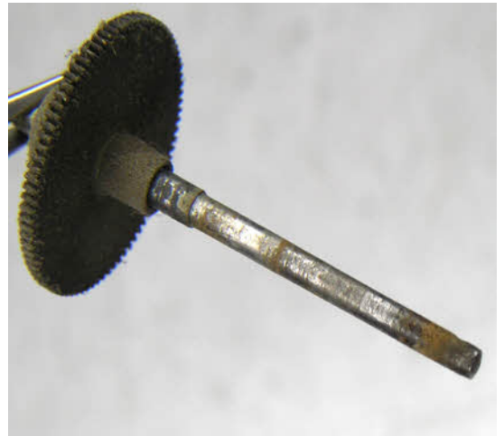
The centre arbour was also tight and had a light rust. It too will clean up well.
