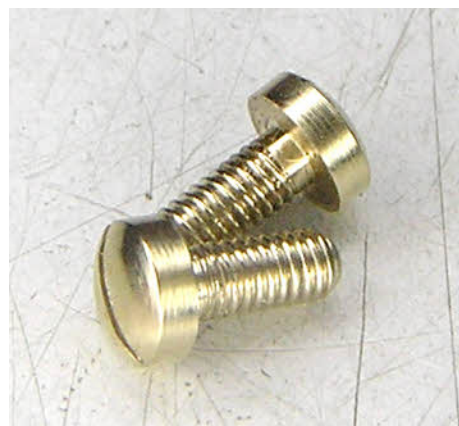
The case parts cleaned and lacquered ready for reassembly. Above are the two new screws turned up to replace the missing ones. These secure the bottom plate to the base via the two threaded inserts.
