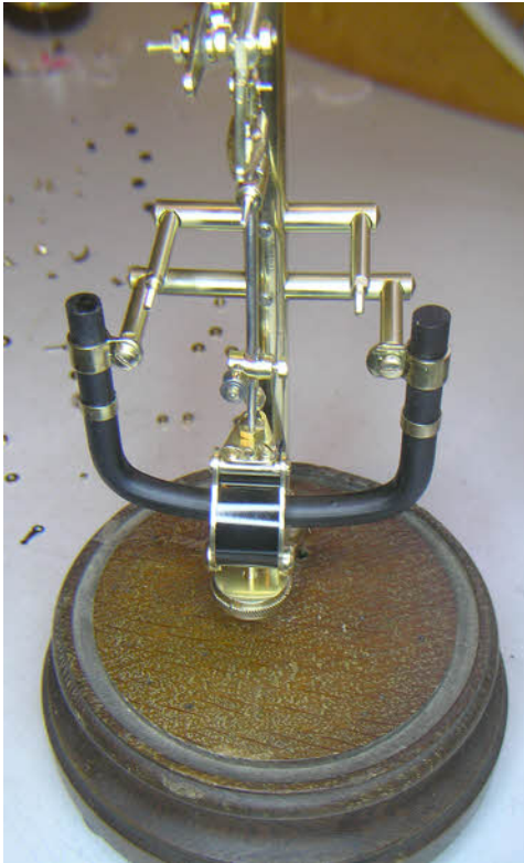
These photos show the frame and pendulum on a old base for testing as well as a couple of shots showing the movement back in place and connected.
