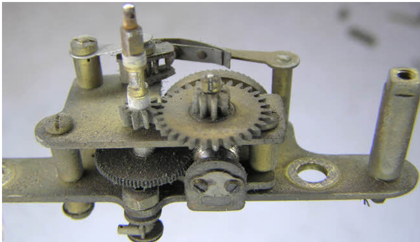
The front and base of the movement. Note the sticky white residue on the canon pinion. The hour wheel was jammed solid with it.
