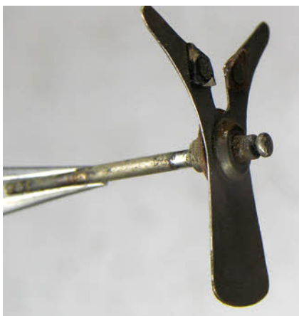
The fork arbour also had a light rust covering but the fork and contacts look in good condition. The photo on the right shows the coil assembly. The casing will need repainting. I normally do any painting and casework before restoring the movement, thus allowing a good couple of days for drying and hardening.
