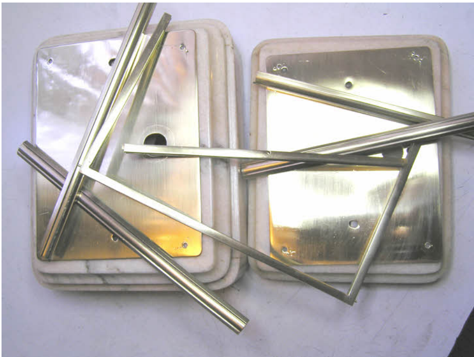
The case parts cleaned and lacquered ready for reassembly. Above are the two new screws turned up to replace the missing ones. These secure the bottom plate to the base via the two threaded inserts.
