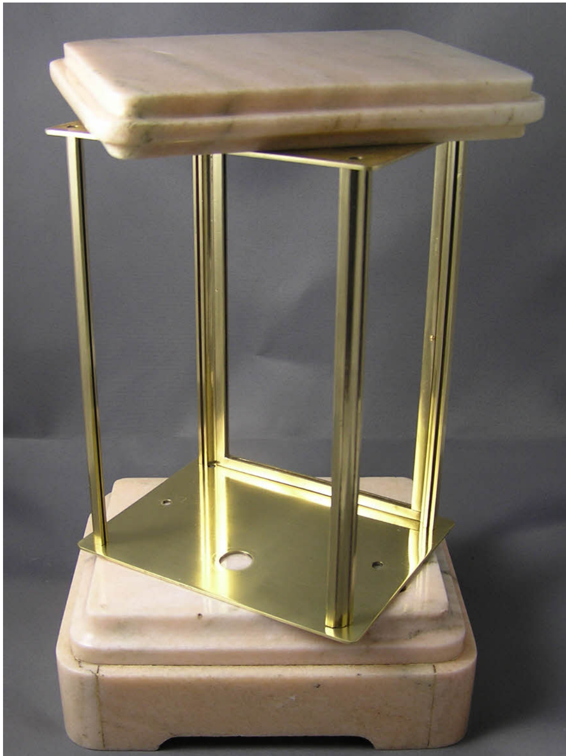
The base, top and brass four glass frame ready to receive the movement.
