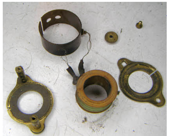
The fork arbour also had a light rust covering but the fork and contacts look in good condition. The photo on the right shows the coil assembly. The casing will need repainting. I normally do any painting and casework before restoring the movement, thus allowing a good couple of days for drying and hardening.
