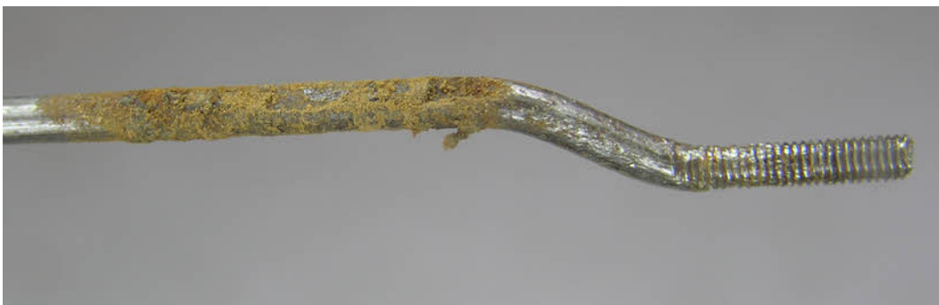
This last photo shows the damage to the steel pendulum rod where the contact pin assembly was heated when soldering the silver pin. It will easily clean up .
