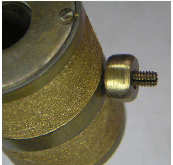
The original rating nut is missing and has a minute replacement. A new one will be made.
