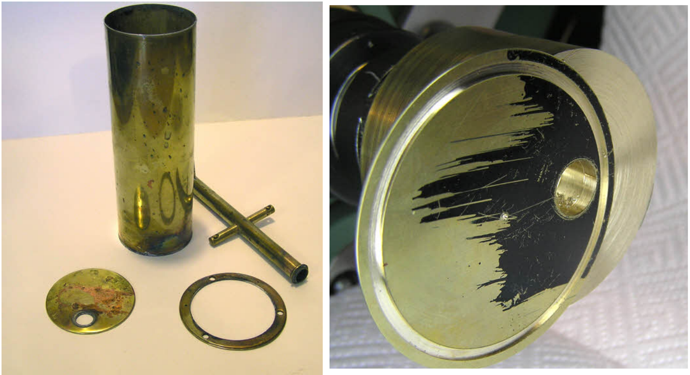
The column, cap and frame disassembled. The last photo shows the new column cap being turned up.
