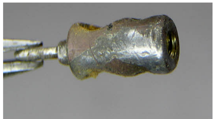
These photos show that the silver contact pin has been soldered in place. It seems from the corrosion that it was soldered in place while still in place in the clock. Hence all the burning and corrosion. Below is the contact pin assembly showing the excess solder.
