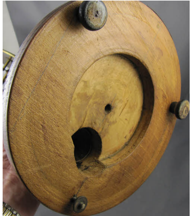
The photo above shows the misshapen hole for the battery holder. There is also no cover.
