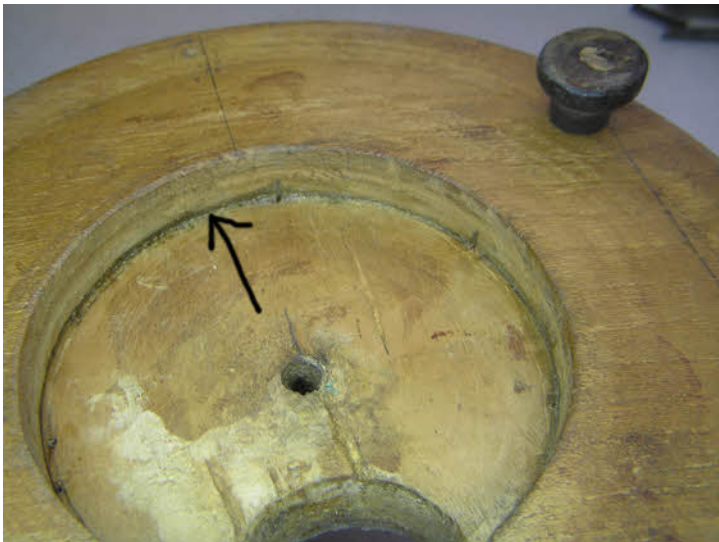
This group of photos shows the base after the column has been removed. The arrows show the two part base and how it has been glued together. Unfortunately the lower parts has warped slightly leaving a larger gap in places at the join.
