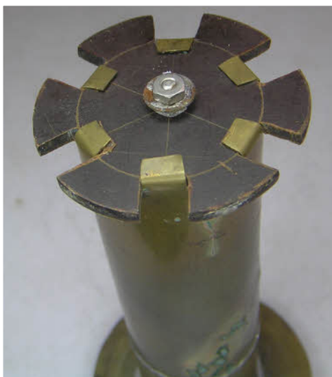
When the column was removed this “battery holder” was found inside. It was also damaged by acid burns. In the photo at top right you can see the colour the base was originally stained.
