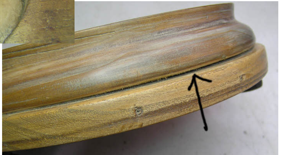
This group of photos shows the base after the column has been removed. The arrows show the two part base and how it has been glued together. Unfortunately the lower parts has warped slightly leaving a larger gap in places at the join.
