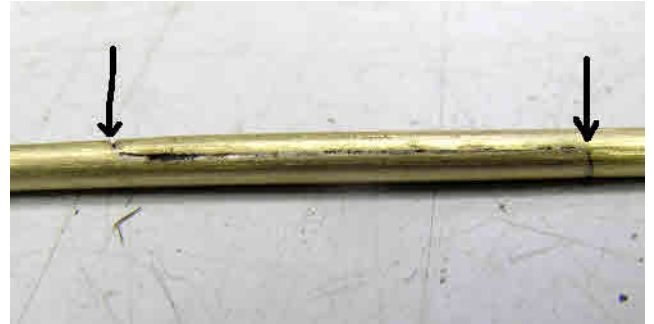
Another made up piece. This is the long brass bar that carries the current from the contact pin down to the coil. Note that it has been soldered in a half housing type joint.
