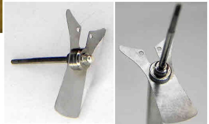
The new collet and fork on the old arbour. The old fork proved to be inconsistent in operation and it was decided to replace it with a more robust and electrically sound fork.
