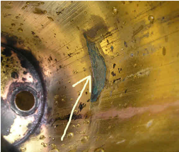
Another made up piece. This is the long brass bar that carries the current from the contact pin down to the coil. Note that it has been soldered in a half housing type joint.
