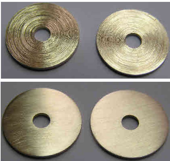
These two photos above show the “engineered” versions (another indicator of major rebuilding) of the dial support washers as found, and after a quick rub with 600 grit...
