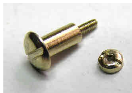
The photo above shows the new pendulum suspension screw and nut. This shouldered screw allows the pendulum to move slightly back and forward to enable it to swing clear of the magnet on a sloping surface.
