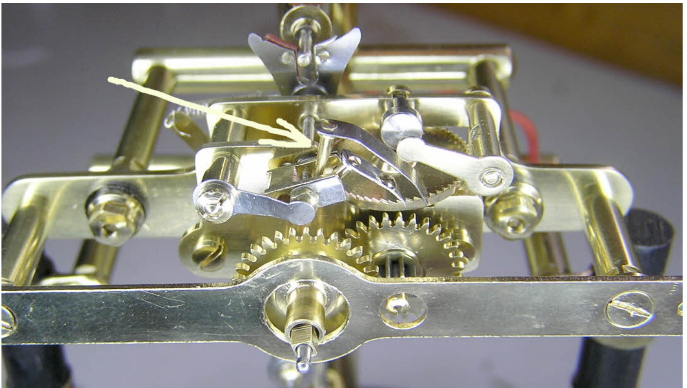
The restored movement back in position. Note the new stop pawl.
