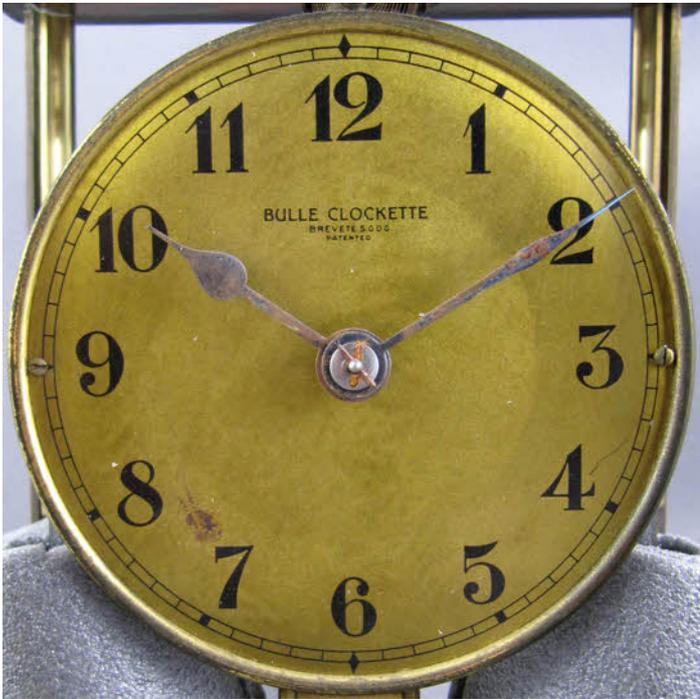
*Above is seen the dial and hands in more detail. Note the rust. Below is a side view of the suspension and movement. All seems OK bar the suspension which has had the ribbon replaced at some time.*
