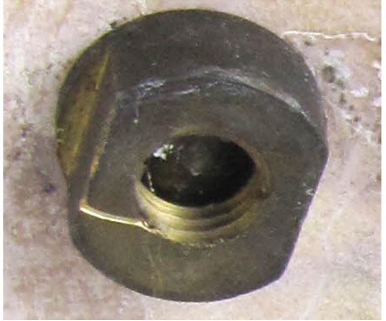
*The underside of the base showing the large nut used to secure the column through the marble. The nut is only secured on a few threads of the column which means that we will have to be very careful when replacing the column to make sure we have enough thread protruding through the marble whilst also taking into consideration the height of the pendulum rating nut as it swings over the magnet. Allowing more thread through the base means less room for the pendulum to swing.*
