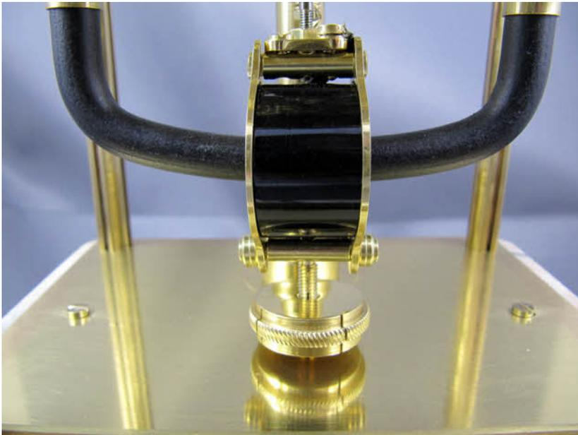
*This photo shows the restored pendulum coil, rating nut and magnet back in position on the marble base.*
