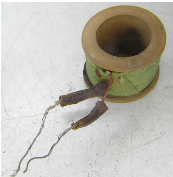
*This group of photos shows the coil with its casing and wax lead wire covers. These wax covers are usually so brittle that they snap and crumble when handled (as in this case). But sometimes they can be reused if heated with a hair dryer every 10 seconds or so before they cool and turn solid.*
