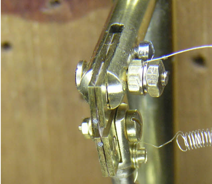
The suspension assembly in place with the correctly positioned contact wire. Note also the suspension mounting slot in the frame has been straightened and tidied up.
