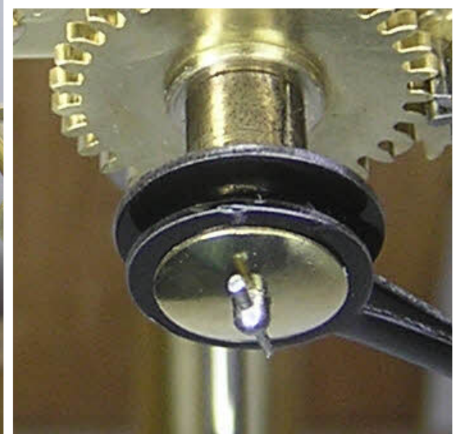
The photo at bottom left shows the movement with hands and collet in place ready for testing. The last photo shows the hand collet in more detail. The pin is centred and a snug fit leaving plenty of metal in the arbour for strength.
