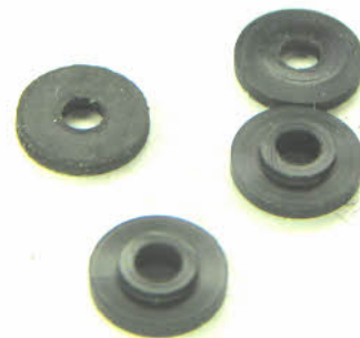
The new set of insulating washers ready to fit.
