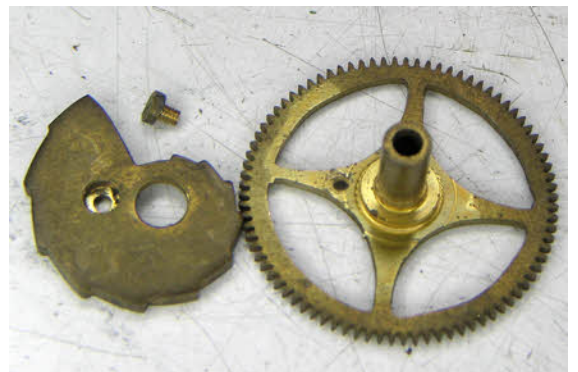
This group of photos shows the motion work and the changes to the movement plate to accommodate them.
