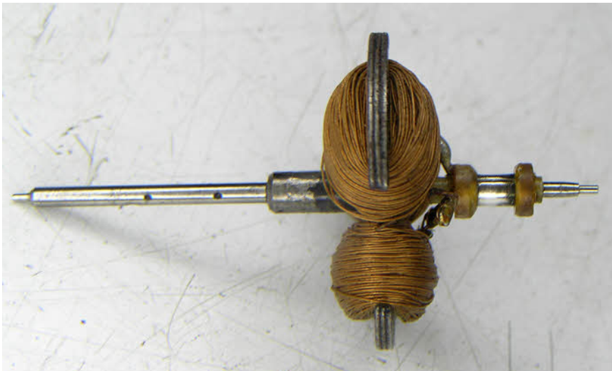
The hammer and rack lift arbour. The two rollers C) sit in the two recesses A) which are enclosed in the shell B) and engage with the square D). The wheel is driven directly by the motor worm wheel.
