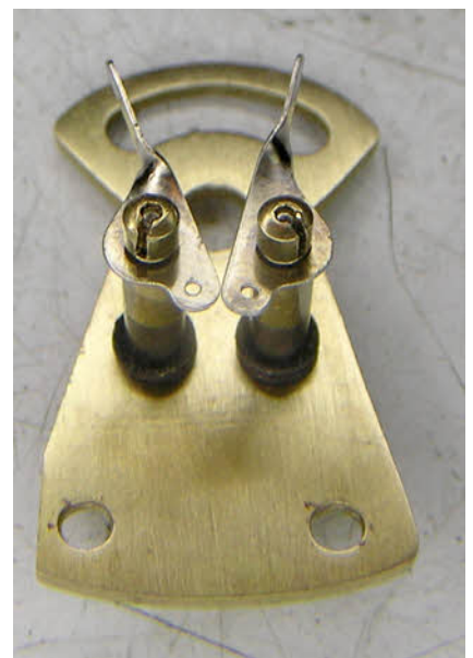
The strike mechanism which has now been completely stripped and cleaned in the ultrasonic tank ready for polishing .
