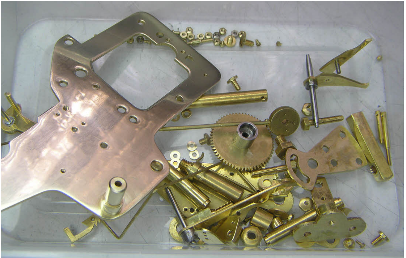
The strike mechanism which has now been completely stripped and cleaned in the ultrasonic tank ready for polishing .
