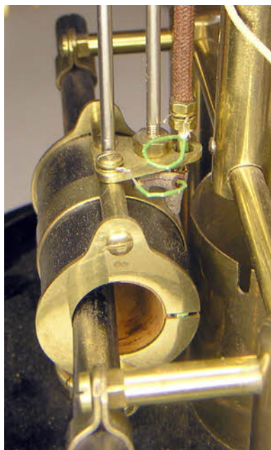
Some shots of the movement and pendulum coil case. Note the wiring which will need checking and insulating when disassembled
