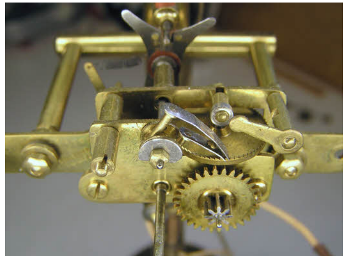
The photo above shows the missing nut from the stud and the missing blued suspension clamping screw. Both will be made and fitted.
