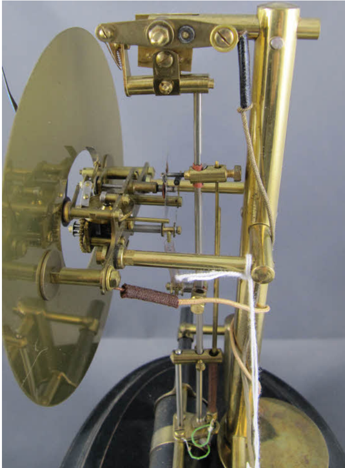
The photo above shows the missing nut from the stud and the missing blued suspension clamping screw. Both will be made and fitted.
