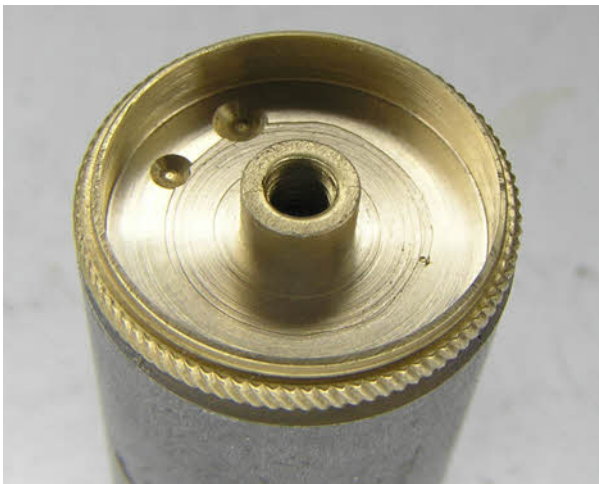
Both the silver and fibre contacts will need replacing.
