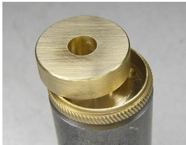
Here we see in more detail the drilled out rating nut.
