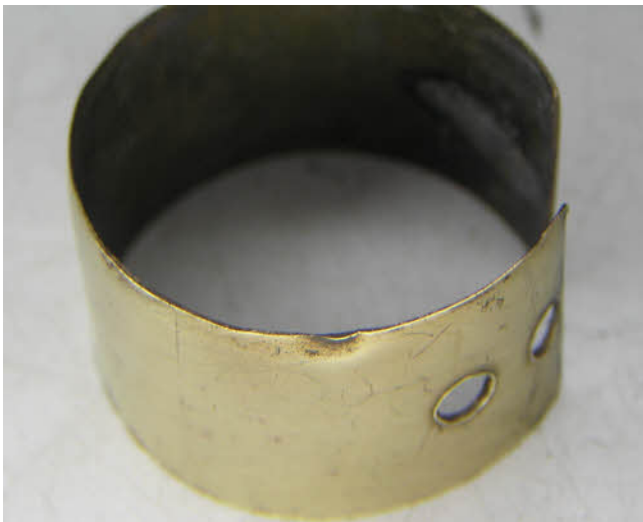
Above we see the slightly damaged coil casing which will be straightened as much as possible before re-spraying.
