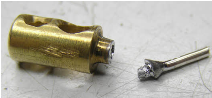
The old pin removed and the new threaded pin inserted.
