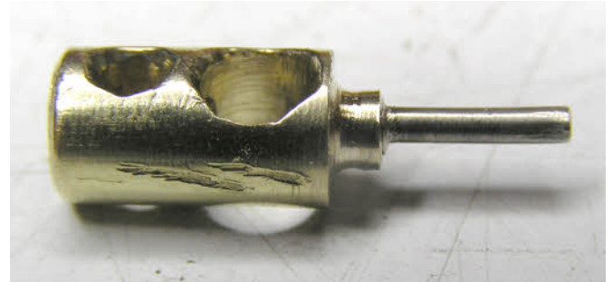
The old pin removed and the new threaded pin inserted.
