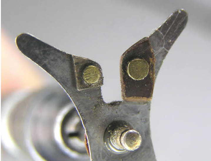
Both the silver and fibre contacts will need replacing.
