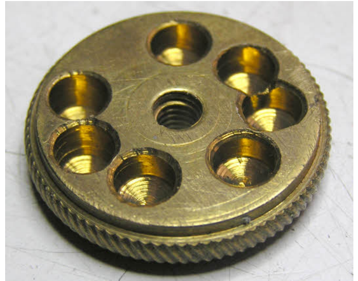
Here we see in more detail the drilled out rating nut.
