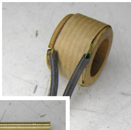
The coil was bound in sticky tape and had single core wire replacing the original. The tape was removed and the coil tidied up and new lead out wire soldered on. The coil was then tested for a normal resistance range of between 1050 and 1250 Ohms.
