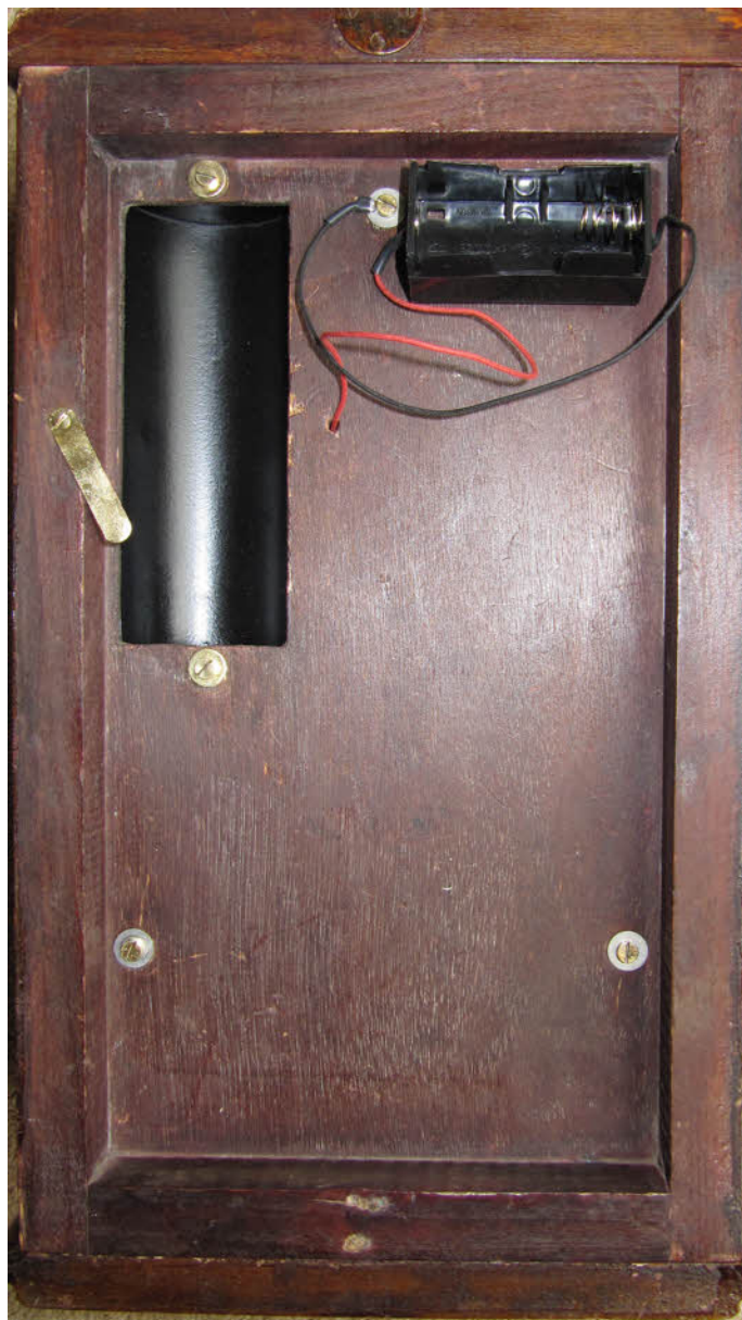
The rear of the clock with restored steel battery compartment.. The battery holder has long terminal leads to allow the battery to be changed easily when the clock is on the wall.
