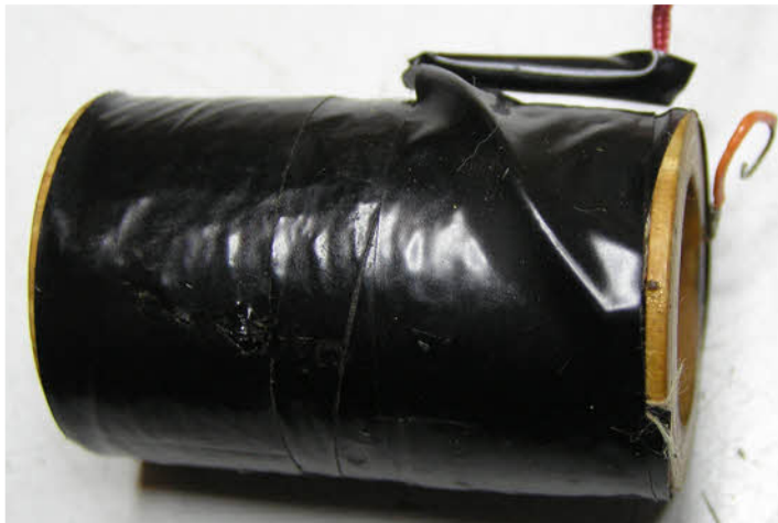
The coil is in a bit of a state. The first lead out from under the coil has obviously broken and has had a new hard single core wire soldered to it. We will try and replace this without damaging it further and necessitating a rewind. The coil itself is bound with modern insulation tape. The good news is that it still shows a good resistance
