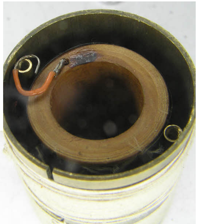
The movement was found to absolutely drenched in oil. The washers will need to be washed and dried, but are still usable
