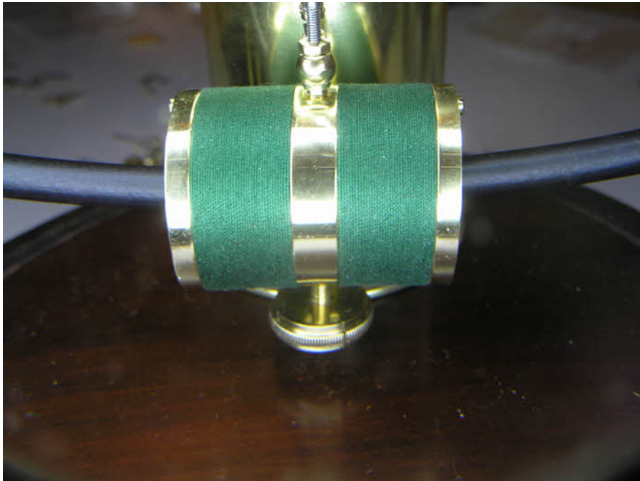
The coil rewound with new cord and back in place with the column and base.
