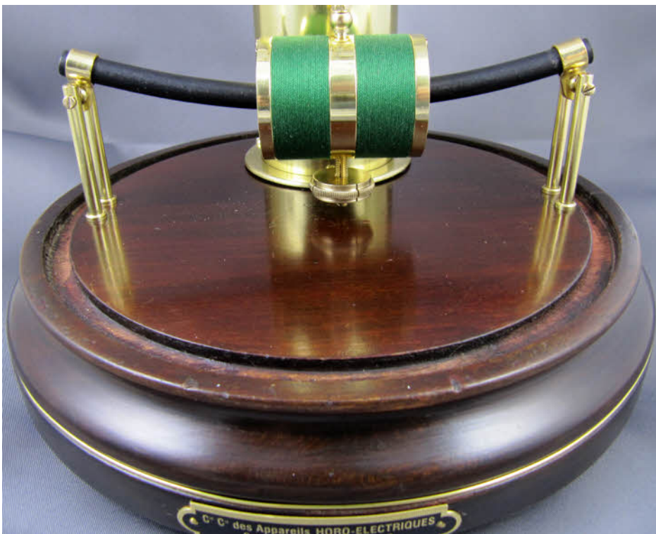
The cleaned movement with new fork contacts back in place.
