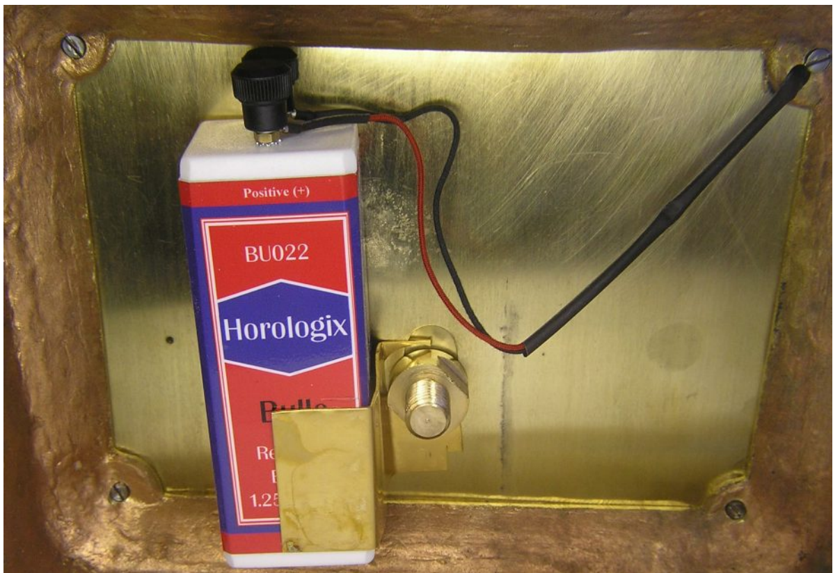
The battery compartment with a Horologix regulated battery fitted. Note the wiring coming through from inside the case after running down the side of the door pillar.
