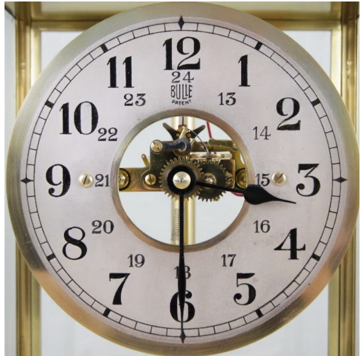
The dial after cleaning and applying silver. Not perfect but a hell of a lot better than when it arrived.
