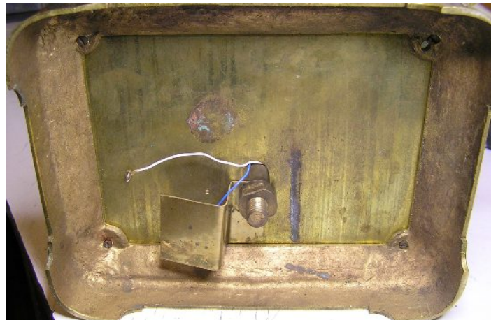
Above is the underside of the base showing the enlarged slot along with a battery retainer. None of this is original. The photo at left shows the missing top retaining screw as well as a steel replacement. A new set will be turned up on the lathe.
