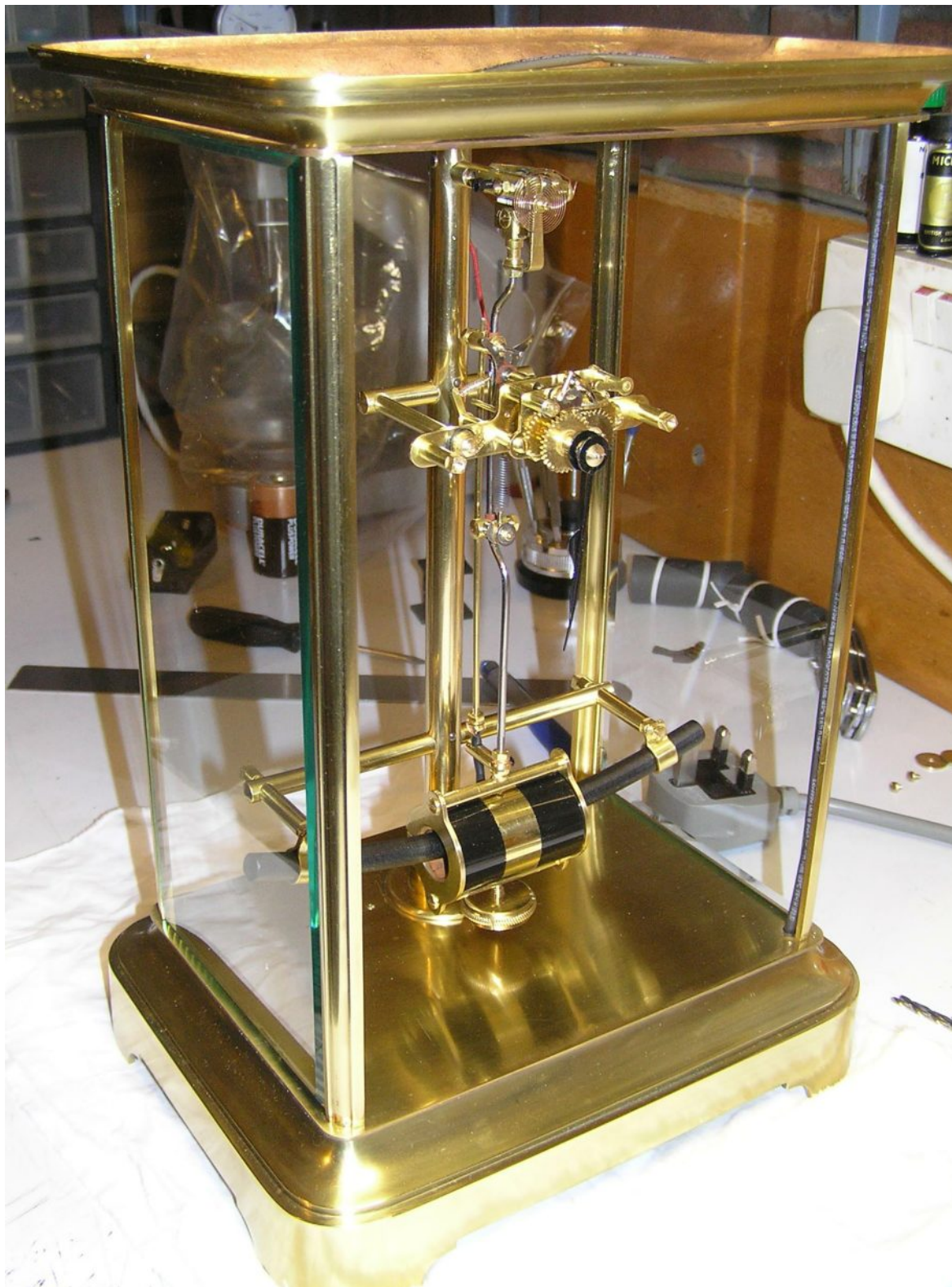
The movement frame installed before the doors and top are finally fitted.
