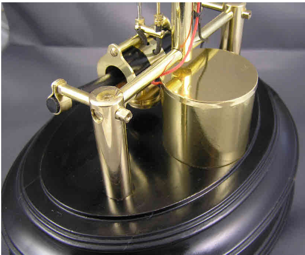
The centre arbour straightened and back in the cleaned movement.
