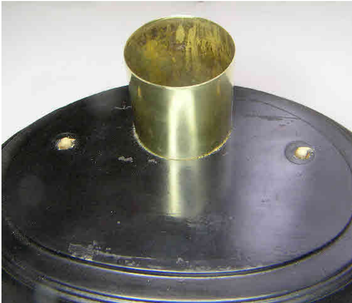
Here the replacement tube can be seen in the newly bored hole in the base.
