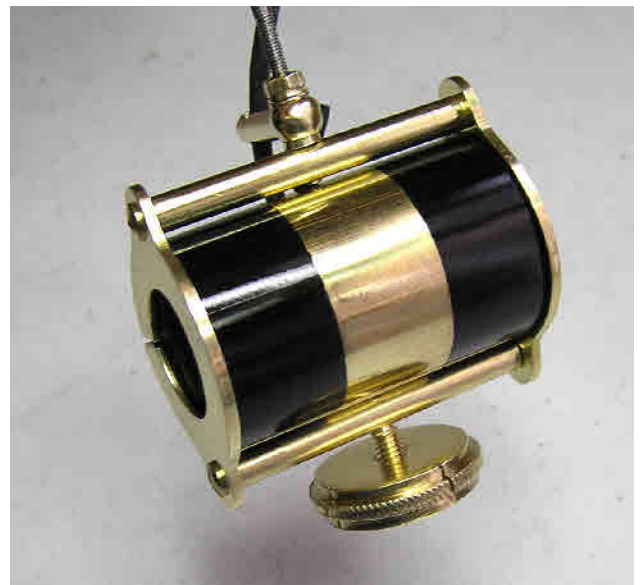
The finished and re-assembled pendulum coil.
