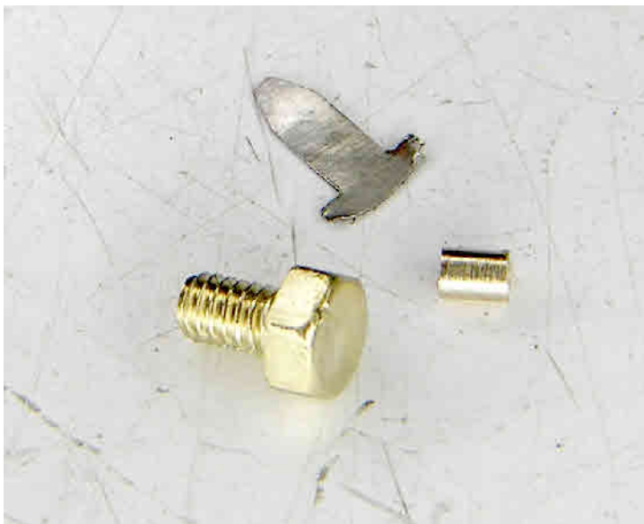
The new contact assembly parts required to complete the pendulum
