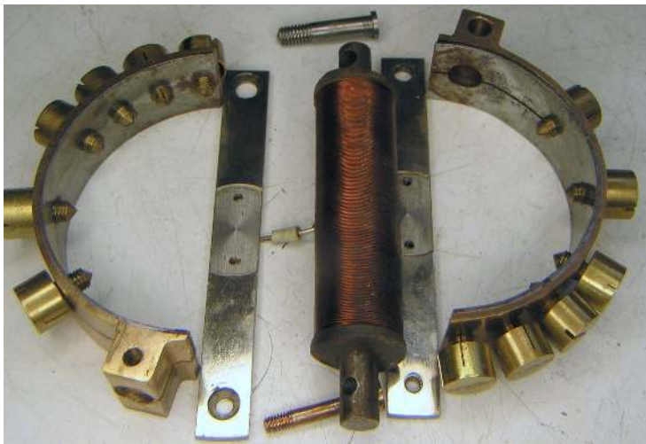
The balance wheel disassembled.
