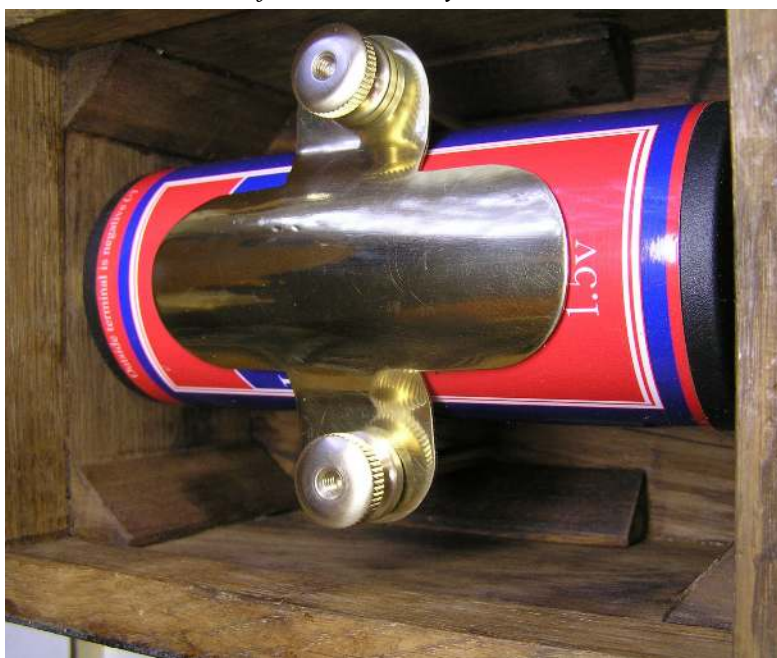
The finished battery retainer.
