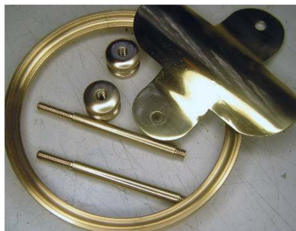
The new parts holding the flag cell battery in place under the base.
