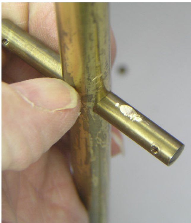
The frame disassembled ready for new rivets which will be turned up on the lathe.
