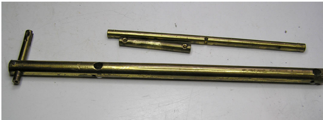
The frame disassembled ready for new rivets which will be turned up on the lathe.
