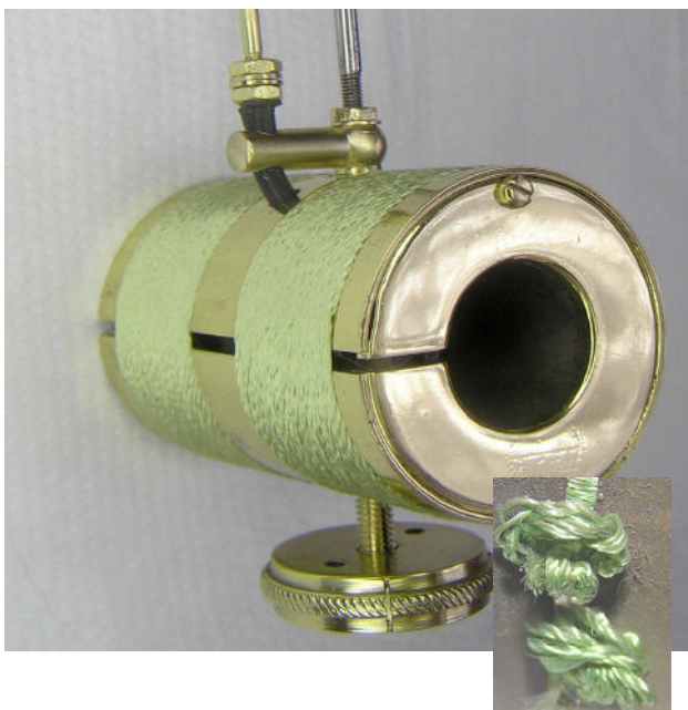
The lower suspension nut and screw were missing and again a new set turned up on the lathe.
