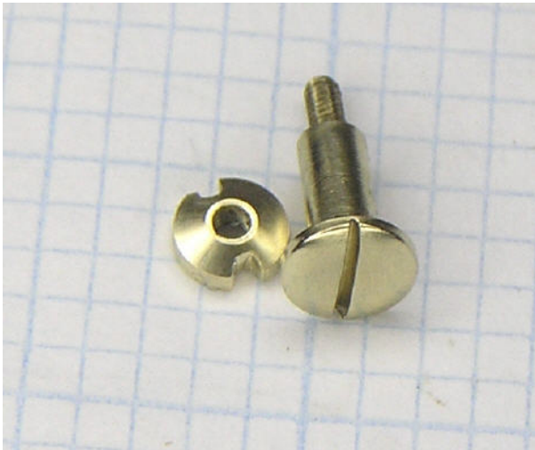
The lower suspension nut and screw were missing and again a new set turned up on the lathe.
